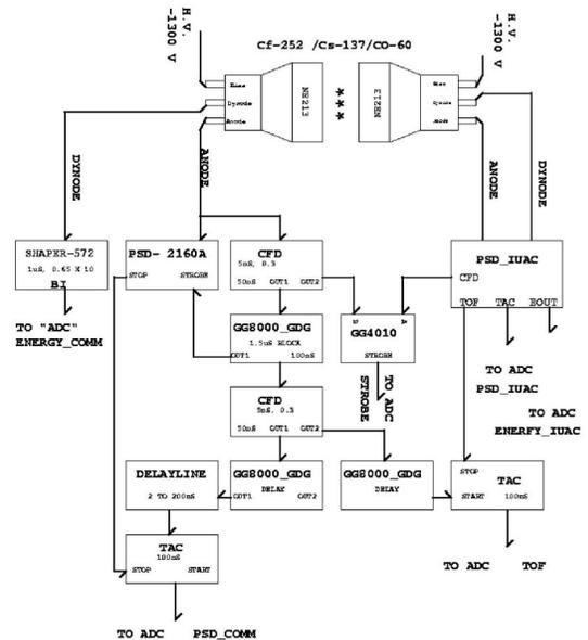
Fig. 7 Test set up for PSD modules
