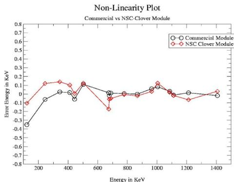
Fig. 5 Linearity plots for Shaping amplifiers
