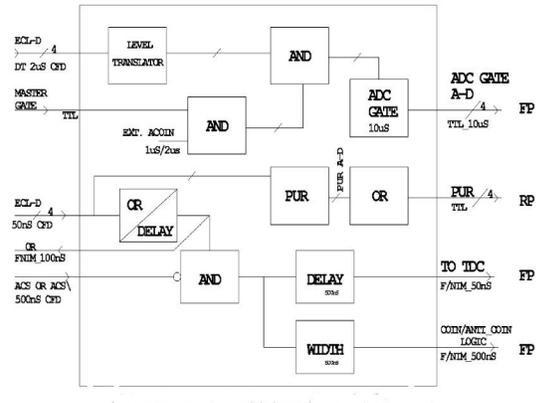
Fig. 3 Block diagram of Anti coincidence logic
