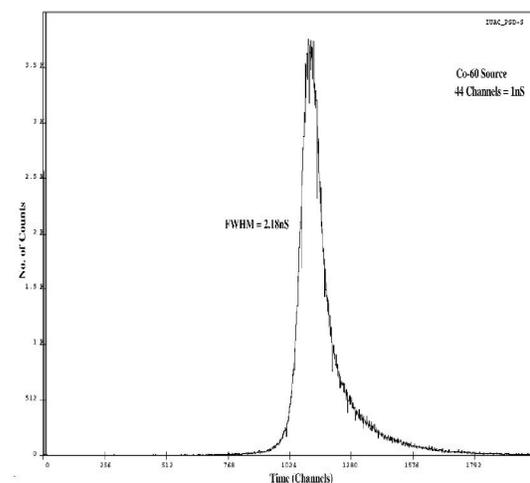
Fig. 9 PSD with  $^{60}\text{Co}$   $\gamma$  ray source
