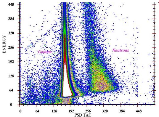
Fig. 11 PSD Vs Energy obtained with  $^{28}\text{Si}$  on  $^{181}\text{Ta}$
