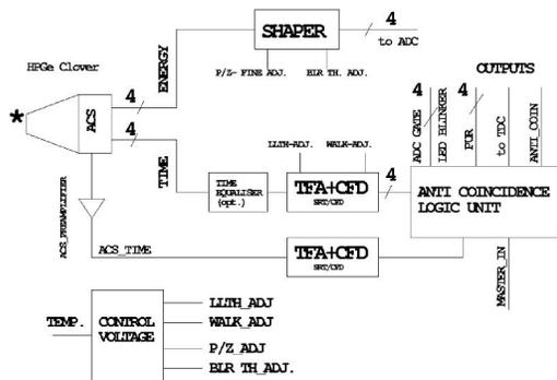
Fig.1 Block diagram of Clover electronics
