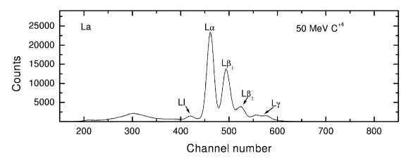
Fig. 1 : L X-ray spectrum of La target at 50 MeV C<sup>+4</sup> beam
