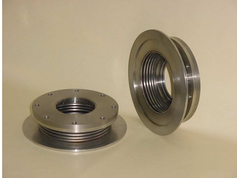
Fig. 5: Modified coupling port transition flange assembly.
