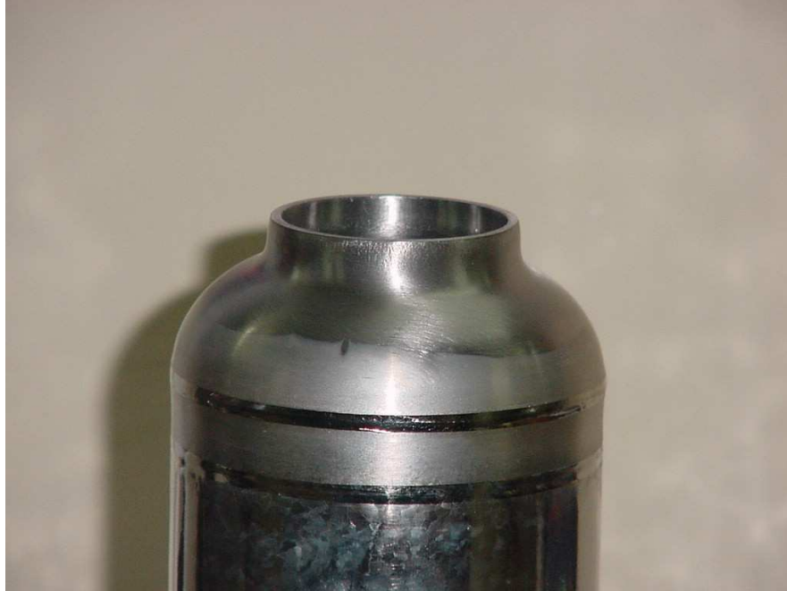
Fig. 9: QWR-6 drift tube after e-beam welding a new upper cap.
