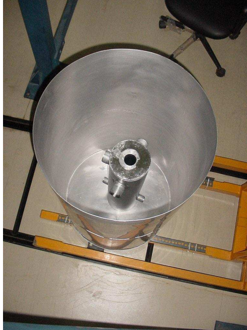
Fig. 4: Niobium Getter box with a resonator loaded in it.
