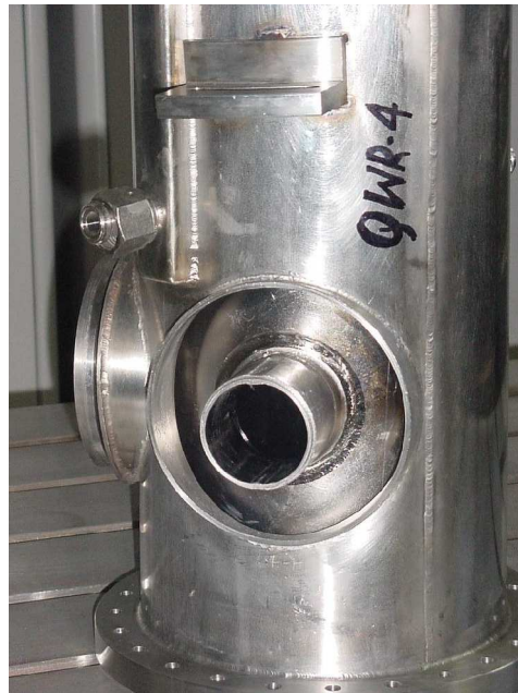
Fig. 5: Modified coupling port transition flange assembly.
