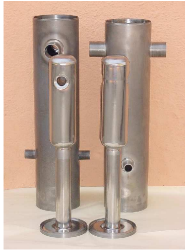
Fig. 3: Niobium outer housing and central conductors of QWR-I2 & I3
