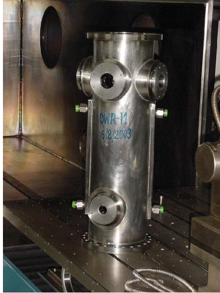
Fig. 1: First indigenously built niobium quarter wave resonator
