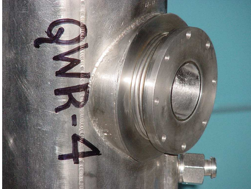
Fig. 7: Coupling port of QWR-4 after installing the modified assembly.
