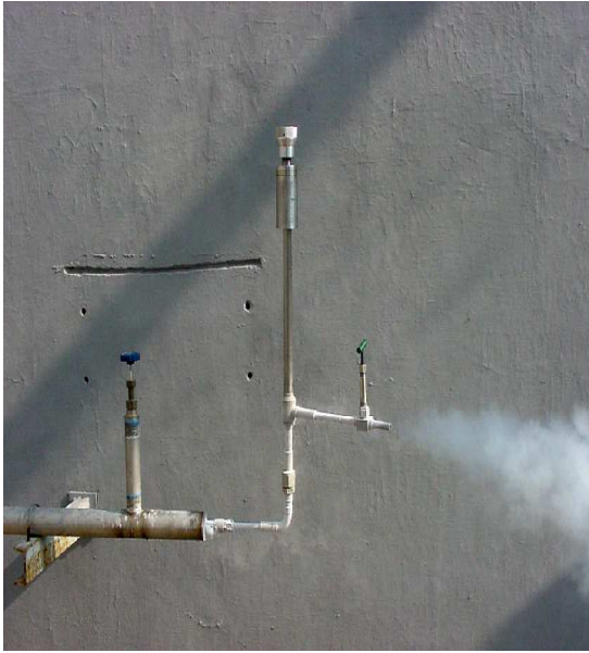
Fig 6 : Cryogenic valve developed at NSC
