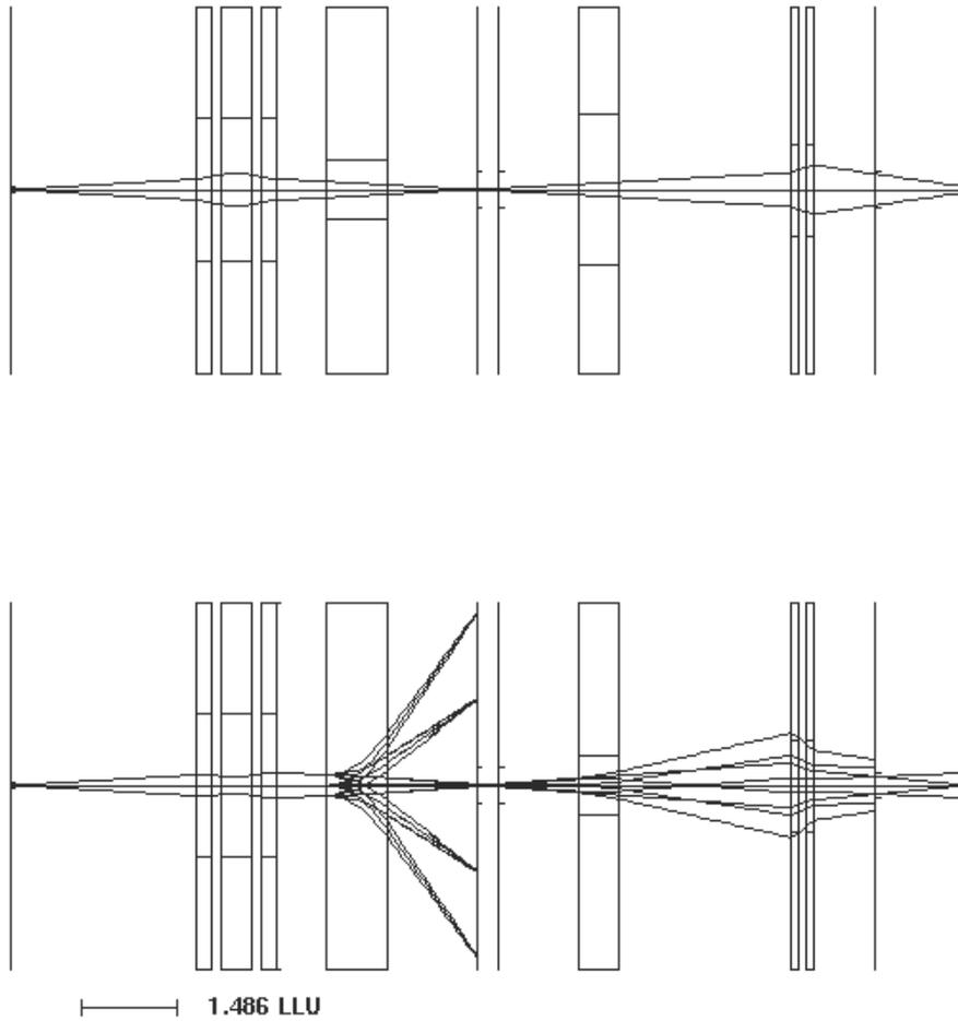
Fig. 1 Beam Optics Calculation with GIOS for AMS beam line. Top part is the Y plane, the bottom part is the x-plane. Major elements shown are the Magnetic quadrupole triplet in vault, Switching magnet, Wien Filter and Quadrupole Doublet, in addition to some apertures. The calculation is for 48MeV,  $^{10}\text{Be}^{3+}$  charge state with mass deviation of 10% and energy deviation of 10%. (i.e. 3 masses and 3 energies)
