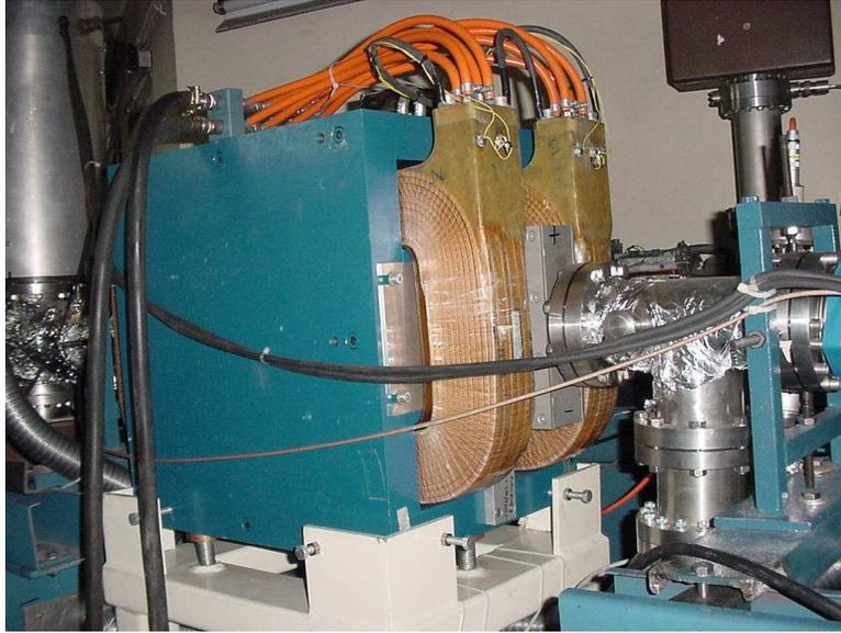
**Fig.3. Wien filter assembly installed in beam line.**
