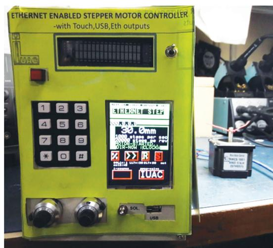
Fig. 3.1.47 Photograph to ethernet enabled stepper motor controller
