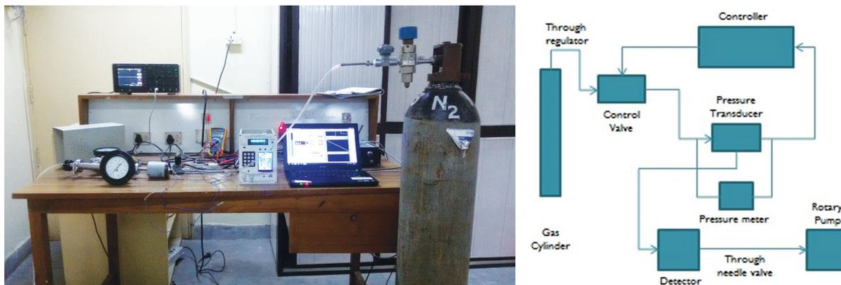
Fig. 3.1.46 (Left) Photograph and (Right) block diagram of PID based detector gas from controller.
