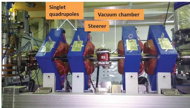
Figure 3.1.1. Quadrupole Singlets of LEBT section
