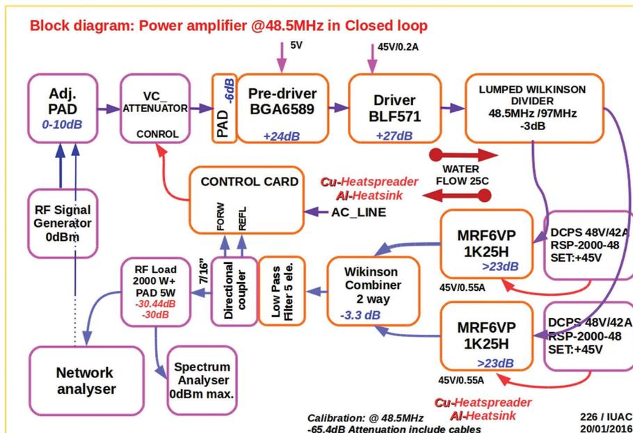
Fig 3.1.32: Block diagram of 2kW, 48.5MHz RF amplifier
