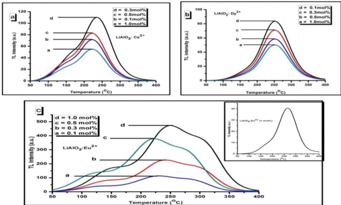
Fig. 3.1.38 TL glow curve for different concentration of a) (0.1-1.0 mol%)  $\text{Ce}^{3+}$  b) (0.1- 1.0 mol%)  $\text{Dy}^{3+}$  c) (0.1-1.0 mol%)  $\text{Eu}^{2+}$  (inset Fig. shows the TL glow of 1mol%  $\text{Eu}^{3+}$  doped  $\text{LiAlO}_2$  phosphor)
