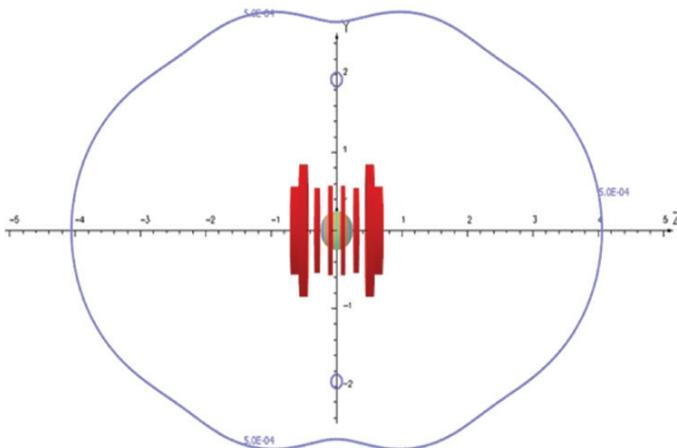
Figure 3.1.18 Iso-homogeneous lines of 2, 4, 6, 8 and 10 ppm homogeneity ; inner most blue line represents 2 ppm and outermost pink line represents 10 ppm [ orange circle represents 45 cm DSV],
