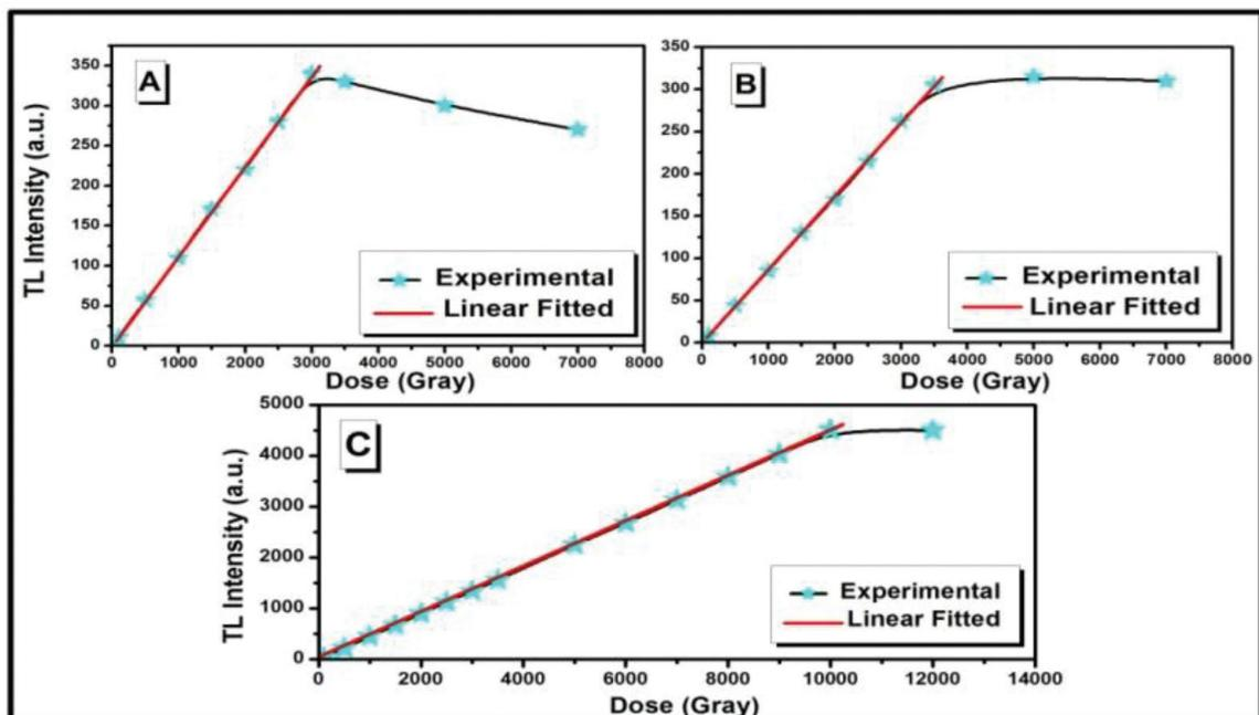
Fig. 3.1.39 TL dose response curve of A)  $\text{LiAlO}_2:\text{Ce}^{3+}$  B)  $\text{LiAlO}_2:\text{Dy}^{3+}$  and C)  $\text{LiAlO}_2:\text{Eu}^{2+}$  phosphors.
