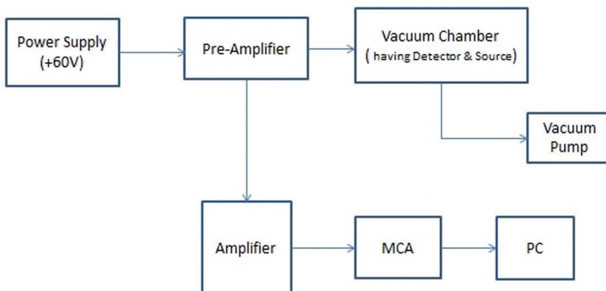
Fig. 3.1.44 Block diagram of new target thickness measurements setup
