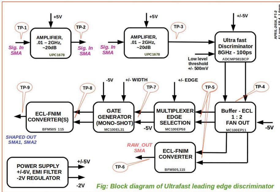
Fig 3.1.31: Block diagram of Ultra fast leading edge discriminator
