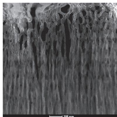
Fig. 3.1.41: Cross-sectional HAADF image showing trenches in anodized alumina
