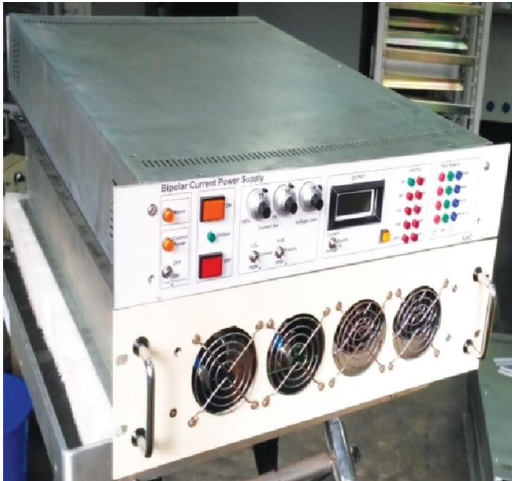
Figure 3.1.25: 25A Bipolar Supply
