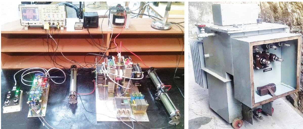
Figure 3.1.27 (a) Laboratory scale fault current generator and (b) step-down transformer
