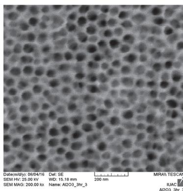
Fig. 3.1.40: Plan-view SEM image showing porous anodized alumina
