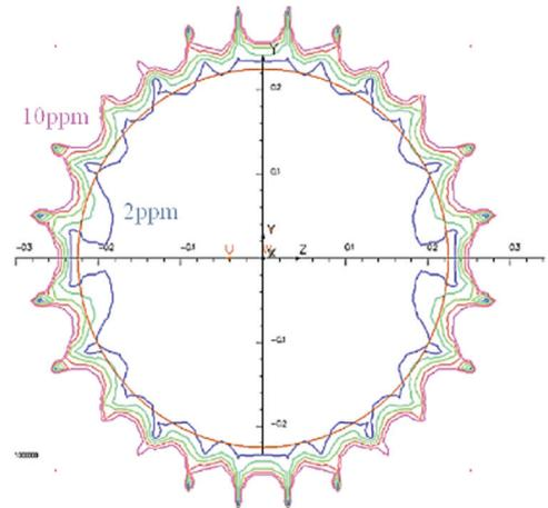
Figure 3.1.19 5G stray field region of the magnet at 1.5T central field. The corresponding peak-to-peak homogeneity is 9ppm.
