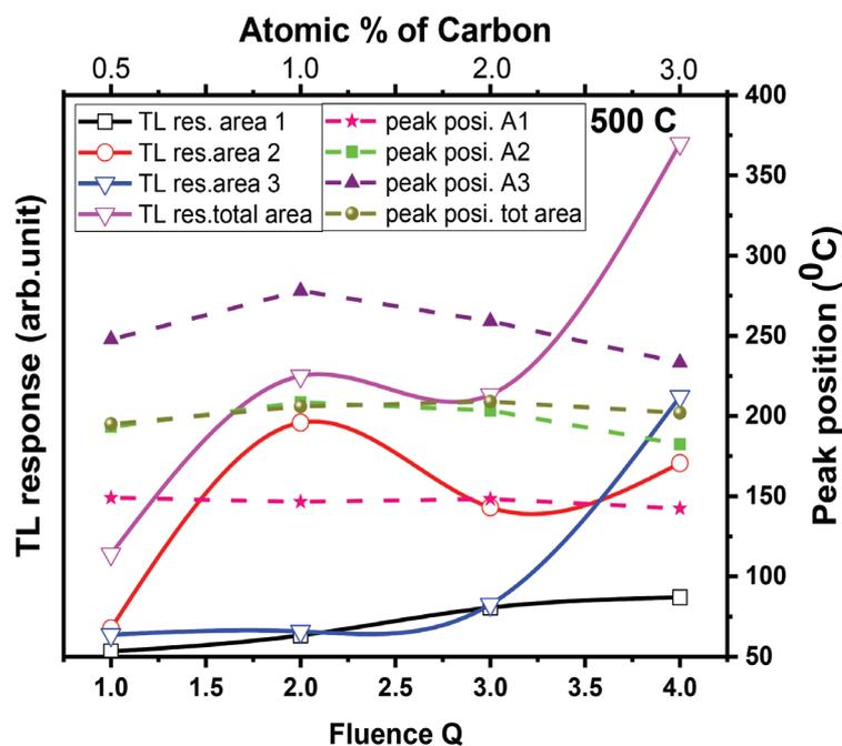
Fig. 3.1.42: TL response (superimposed with fitted data) after  $C^+$  implantation with various fluences ( $Q$  in ions/cm<sup>2</sup>).
