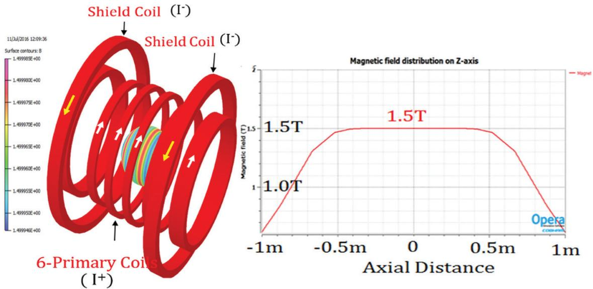
Figure 3.1.17 Multi-coil configuration of 1.5T MRI magnet and its axial field profile.
