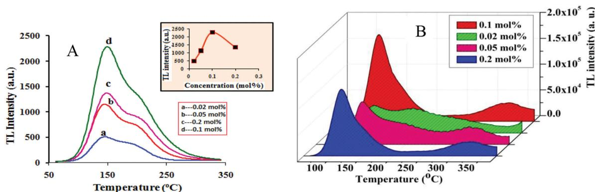
Fig. 3.1.37(A) TL glow curves of  $LiCaBO_3:Cu$  phosphor exposed to 1.2 rad  $\gamma$ -ray exposure, (B) TL glow curves of  $C^{5+}$  ion beam irradiated  $LiCaBO_3:Cu$  phosphor exposed for  $3.75 \times 10^{12}$  ion  $cm^{-2}$ .
