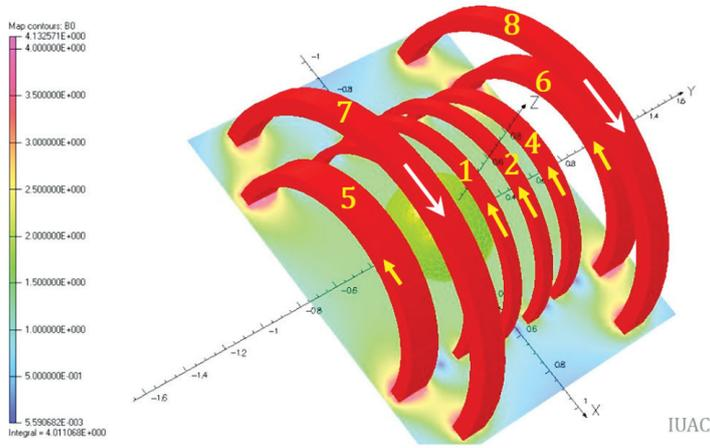
Figure 3.1.20 The field concentration on different coils of the 1.5T MRI magnet.
