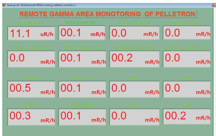
Fig. 3.1.36 Remote readout facility panel
