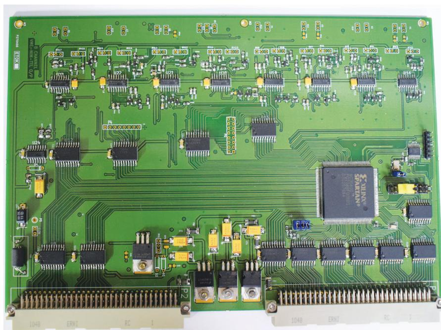
Fig. 3.1.43 The module can be used in VME based data acquisition for generating BUSY I/O signal.
