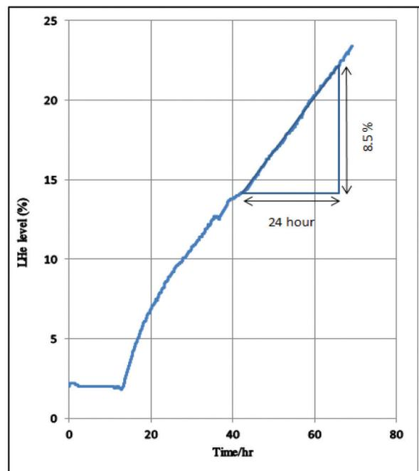
Figure 3.1.22 GM Cryocooler liquefier and its liquefaction rate
