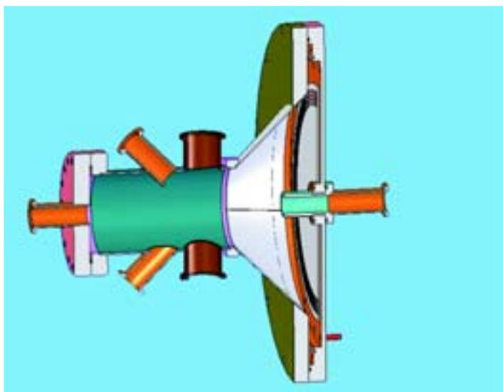
**Fig. 1. Large area position sensitive annular PPAC**
