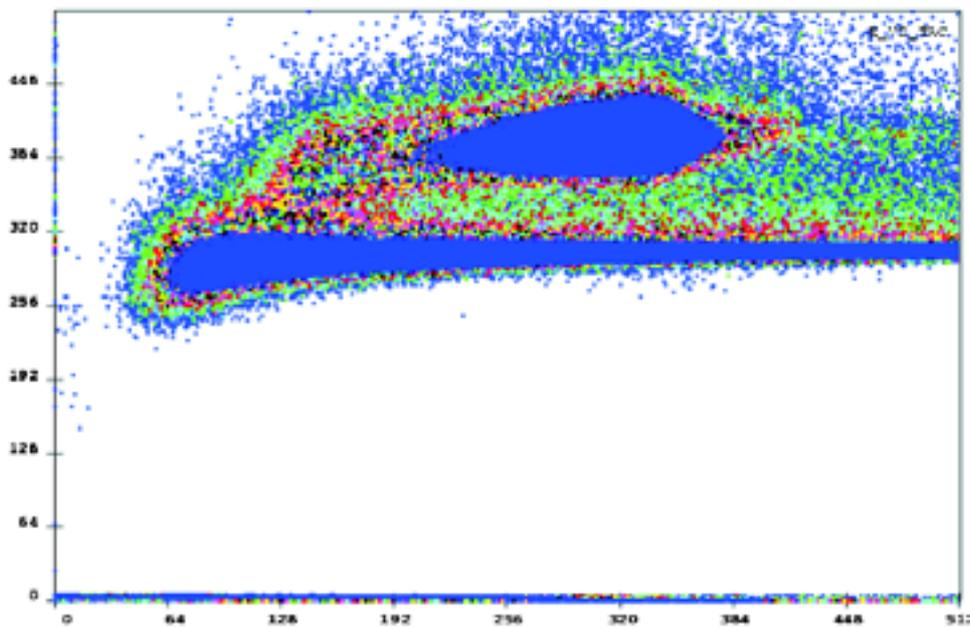
**Fig. 2. Gamma and alpha particle discrimination using zero-cross method using CsI+PIN detector.**
