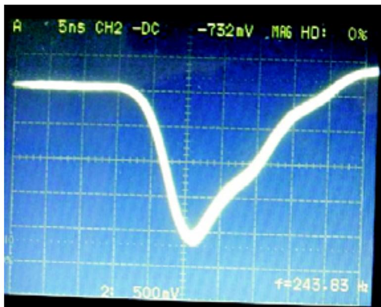
**Fig. 3. Output pulse from pre-amplifier for silicon detector and alpha source**
