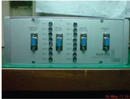
Fig. 9. The Picture of WEB-PLC
