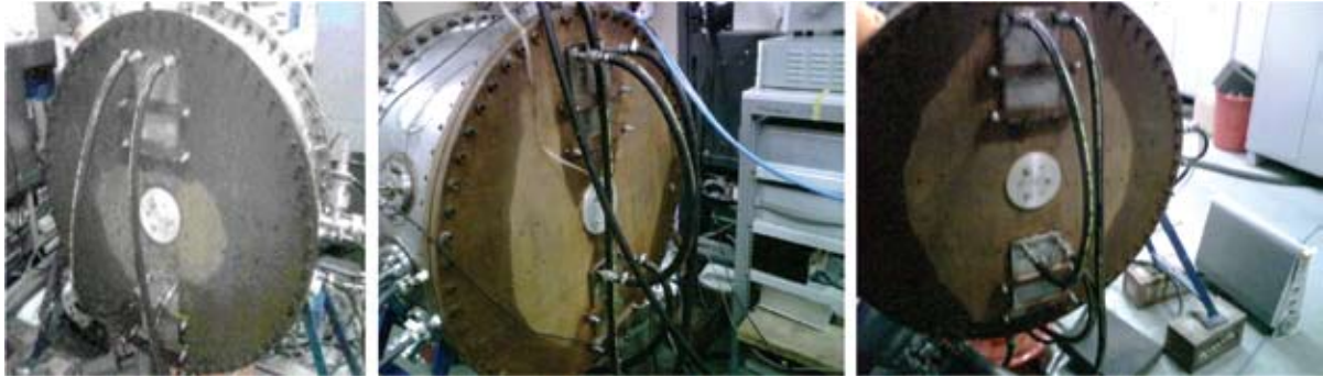
Fig. 6. Heating Effect as Seen on End Plates at 3 kW, 4 kW and 6 kW
