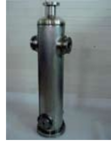
Fig. 2. First prototype niobium low beta resonator built at IUAC.
