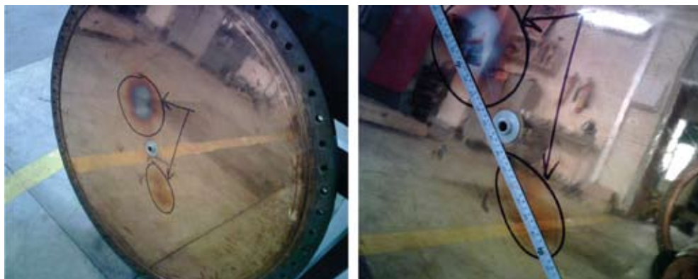
Fig. 1. Multipactoring Effect on the Exit Flange
