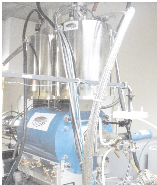
Fig. 1 : HTS ECR ion source with the extraction system (extreme left).
