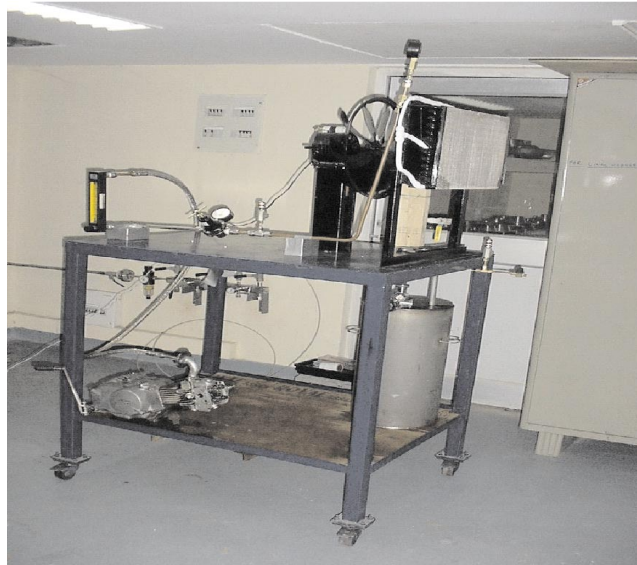
Fig. 7 : LN 2 driven prime mover
