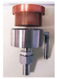
Fig 7. The heat exchanger block of recondenser
