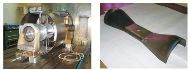
Fig. 4. (a) Left, an Outer Shell setup for electron beam welding, and (b) Right, a Half Spoke formed in niobium.
