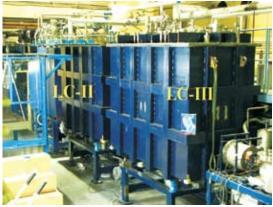
Fig. 5. The IInd and IIIrd Linac cryomodules in the Linac beam line
