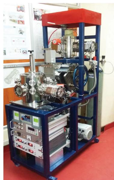
Fig. 1.6.2 IUAC's 30 kV Tabletop Accelerator
