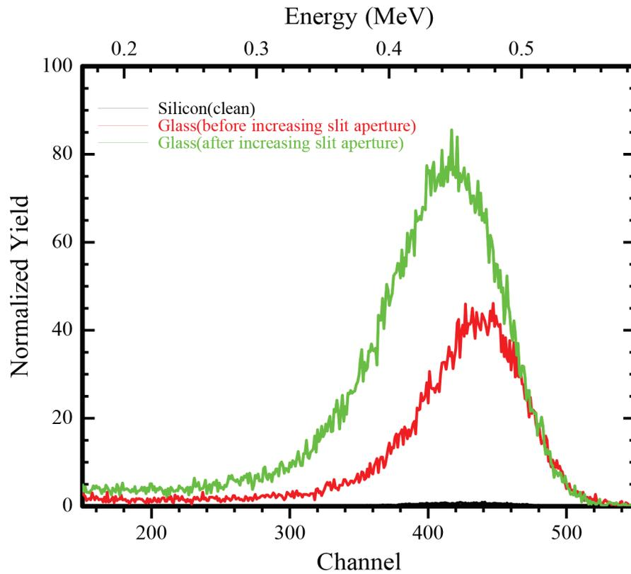
Fig 1.4.1 ERDA spectrum of Au(H) on SiO<sub>2</sub> for two different detector aperture compared with ERDA spectra of cleaned Si.
