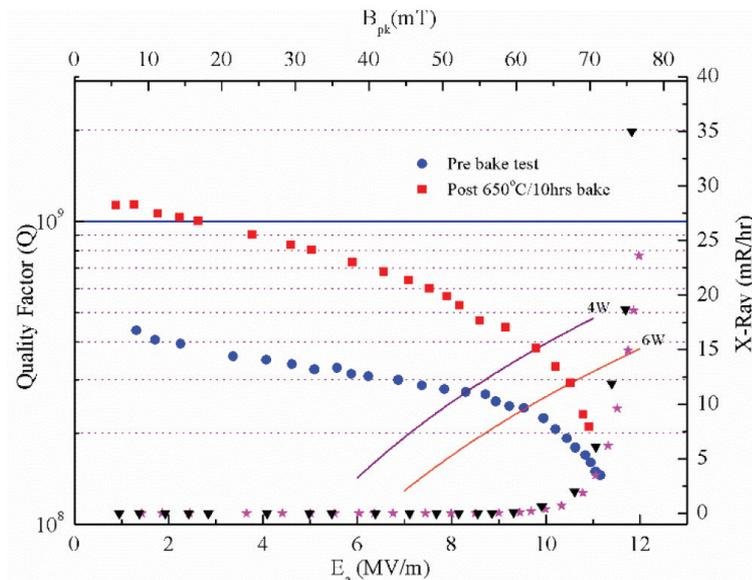
Figure 1.2.4: Q curves for the low beta resonator (LBR) pre and post 650°C bake.
