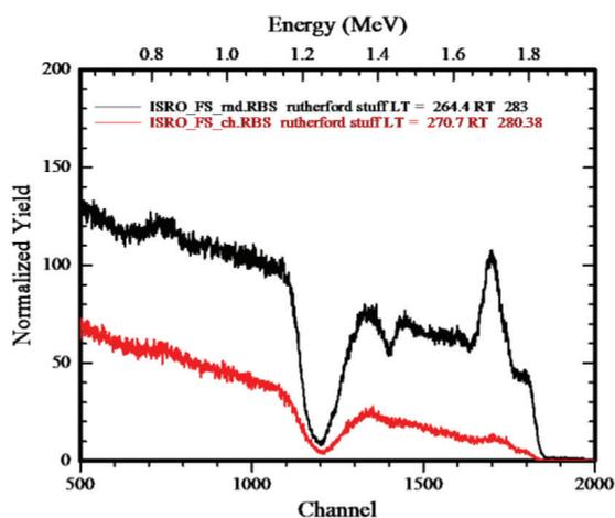
Fig 1.4.4 RBS channeled spectra of Multi-junction solar cell (red) compared with random spectra (black).
