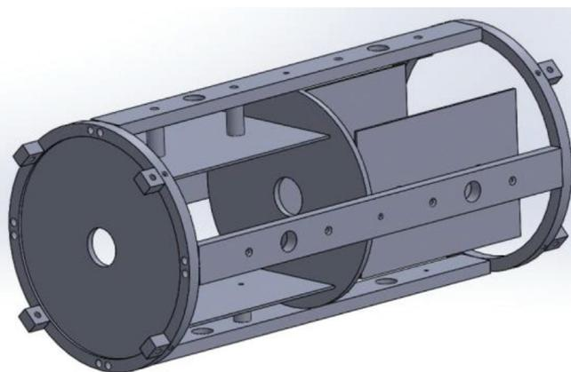
Figure 1.3.4 The inner part of the electrostatic steerer
