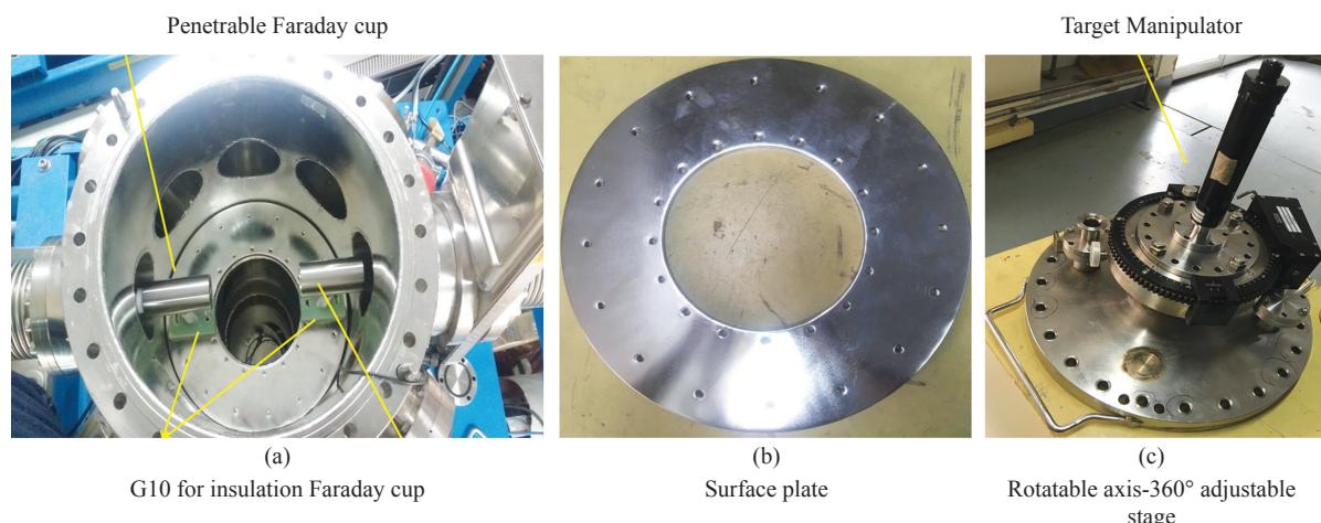
Fig 1: (a) Both the Faraday cups inside vacuum chamber are mounted on the surface plate, (b) surface plate and (c) target manipulator on a rotatable axis-3600 adjustable stage.
