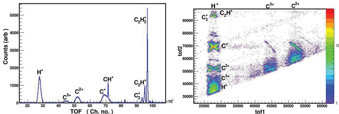
Figure 3: Time of flight spectrum (left) and double ion coincidence spectrum (right) generated in 1.8 MeV Ar<sup>9+</sup> impact on C<sub>2</sub>H<sub>2</sub>
