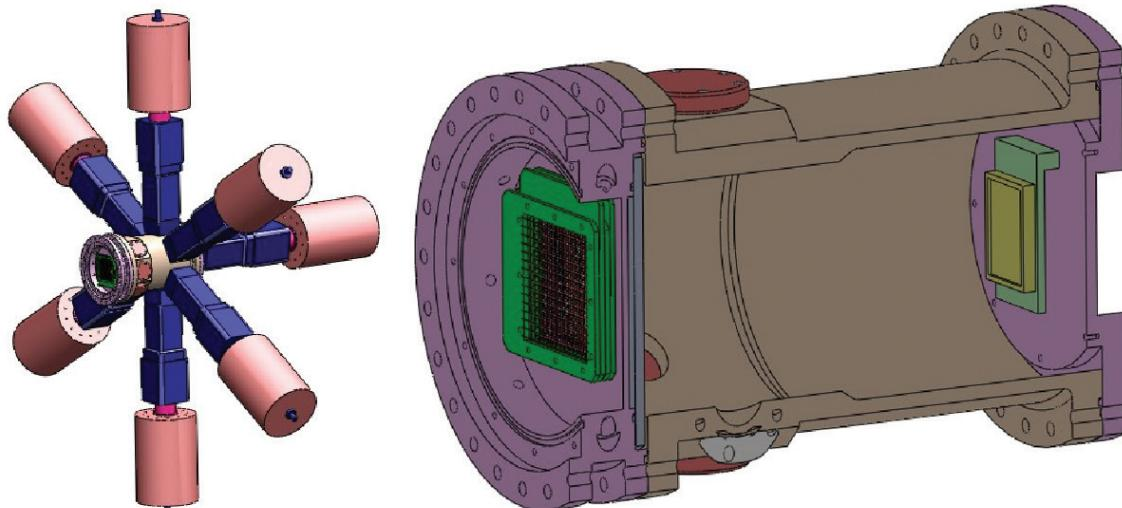
Design of new focal plane detector chamber
