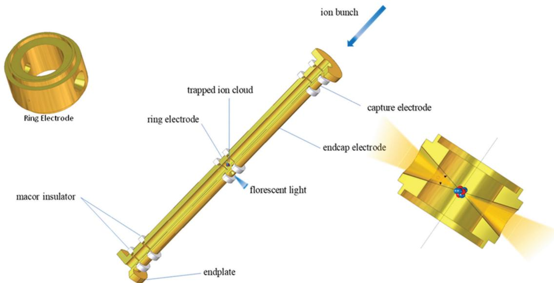
Figure 2: Section view of the ion trap electrodes assembly and ring electrode
