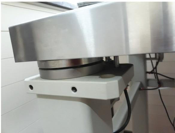
Figure 3: Vibration Isolation Table with adjusting screws
