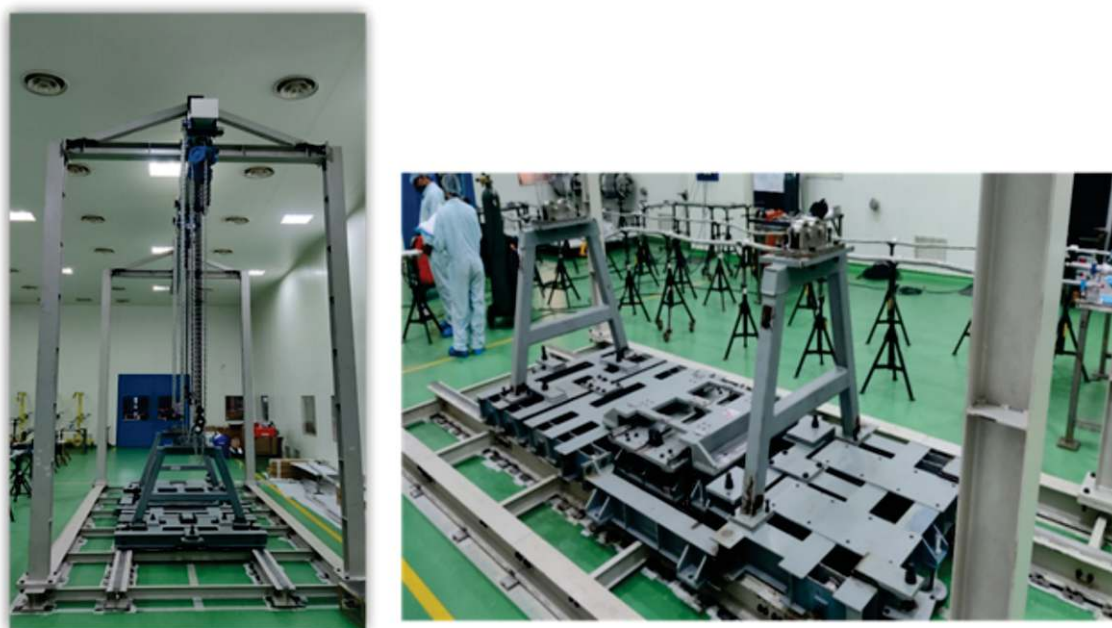
Fig. 3.8 The magnet-cryostat assembly station of the whole-body MRI magnet system.
