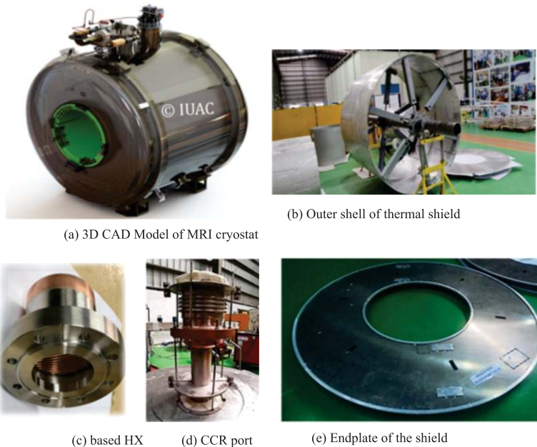
Fig. 3.6 Various components fabricated for the zero-boil-off MRI cryostat.
