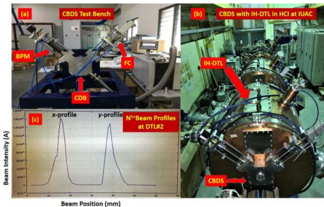
Figure: (a) CBDS offline test bench (b) CBDS installation at the entrance of DTL cavities in HCI and (c) beam profile at the entrance of DTL2 during beam test run in HCI.
