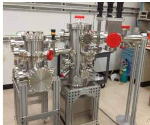
Figure 4. The schematic of the Photocathode Deposition Mechanism with the image of the deposition systems
