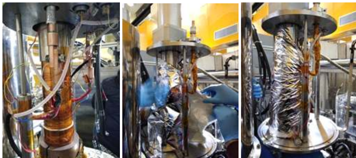
Fig.1 'High current feedthroughs' and 'aluminium-mylar' layers installation
