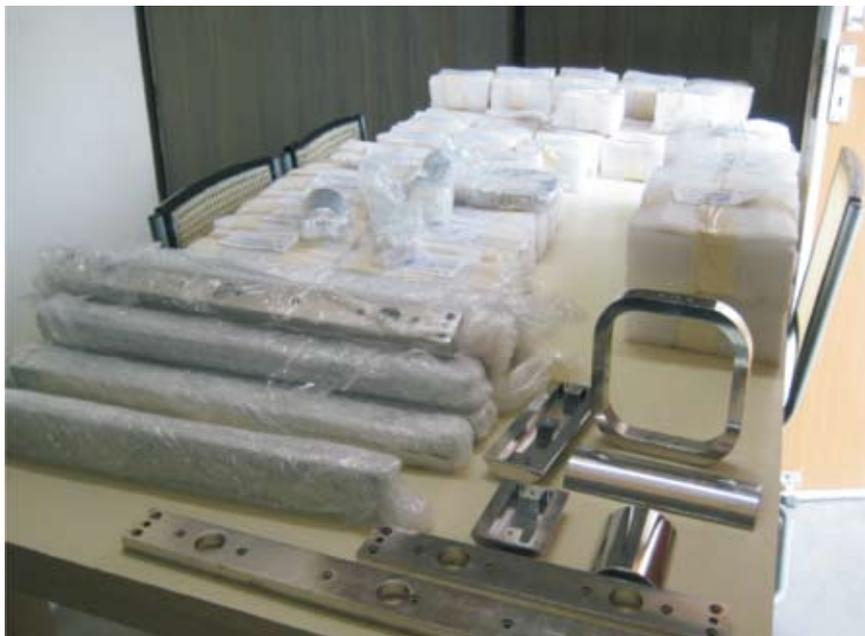
**Fig. 5. Electrostatic Quadrupoles inner components after fabrication**
