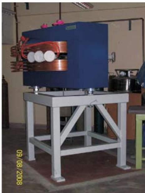
**Fig. 1. Switching Magnet**
