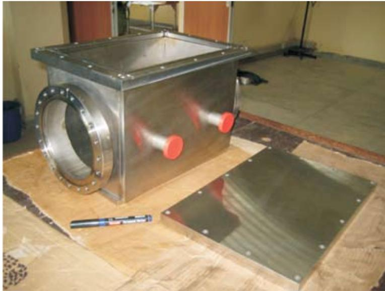
**Fig. 6. Chamber for the gas cell absorber**
