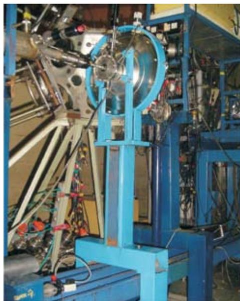
**Fig.2. Annular PPAC setup mounted in GDA beam line**
