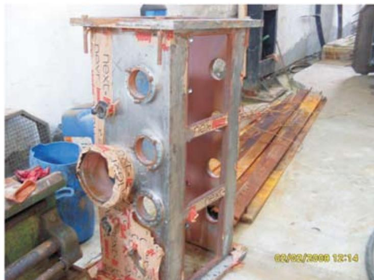
**Fig. 3. Various stages of Copper electro-plating of RFQ chamber**
