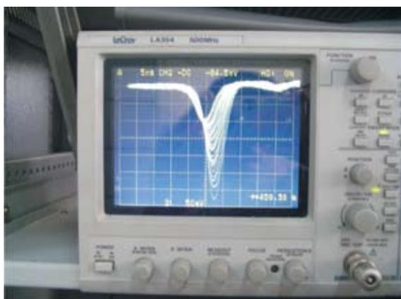
**Fig.3. Timing signal from the cathode preamp (alphas from 241 Am)**
