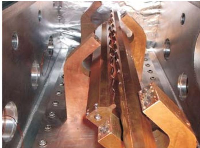
**Fig.1. Assembling of modulated vanes**
