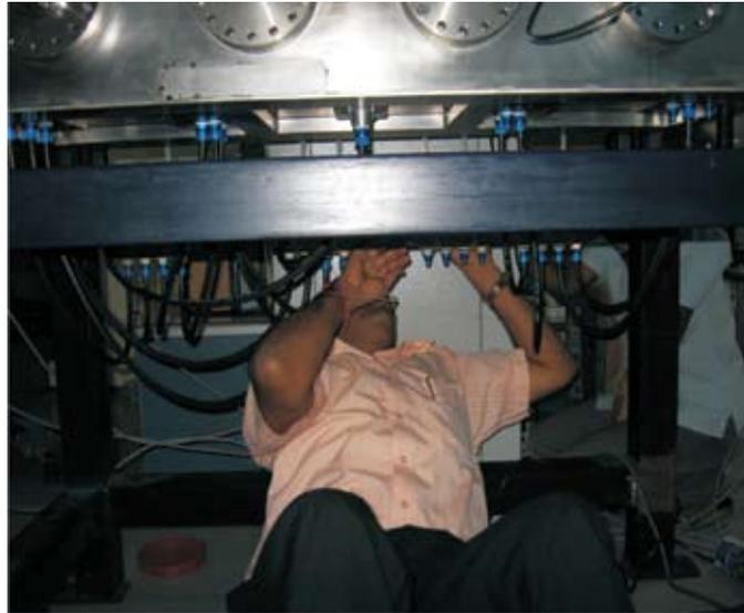
**Fig.2. Assembling of water cooling accessories in progress.**
