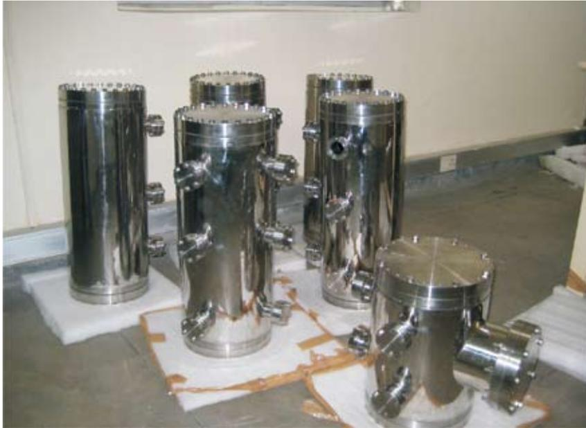
**Fig.4. Electrostatic Quadrupoles UHV chambers after Fabrication**
