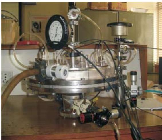
**Fig.1. Annular PPAC during off line test in Detector Laboratory**
