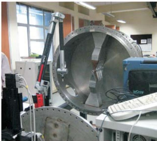
**Fig.12. DTL parts are being assembled and tested.**
