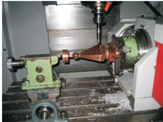
**Fig.10. Stem machining in progress**
