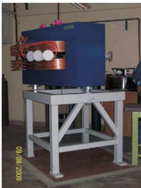
**Fig. 1. Switching Magnet**
