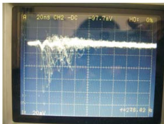
**Fig.4. Delay line position signal triggered by cathode (fig.3)**
