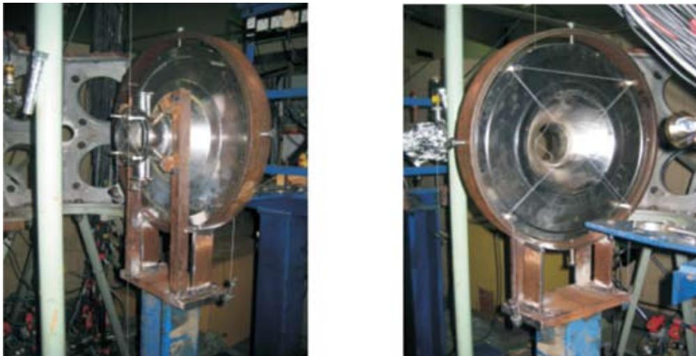
**Fig.7. Conical target chamber for GDA with stand and foil flange**
