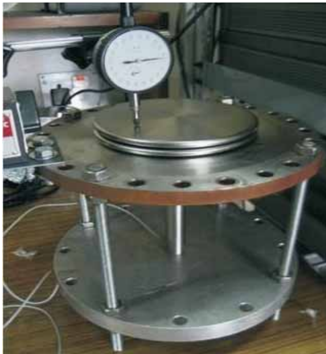
Fig. 2. Measurement of the deflection of niobium bellows after powering the piezoelectric actuator
