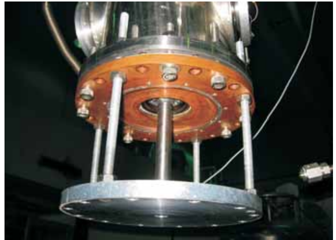
Fig. 3. The mechanical tuner (hiding inside the resonator) along with the piezoelectric actuator prior to a cold test
