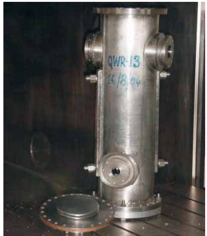
Fig. 1. Niobium quarter wave resonator with slow tuner bellows at IUAC
