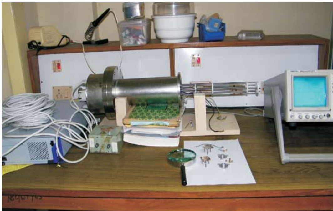
Fig.1. New Plunger for INGA; Foil holders and the cones could be seen in the foreground
