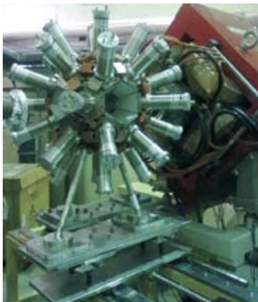
Fig. 2. Spin spectrometer and support structure at HYRA target site
