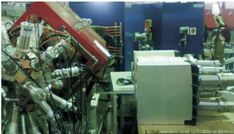
Fig. 3. HYRA gas-filled stage coupled with spin spectrometer and HIGRASP high energy gamma ray detection system
