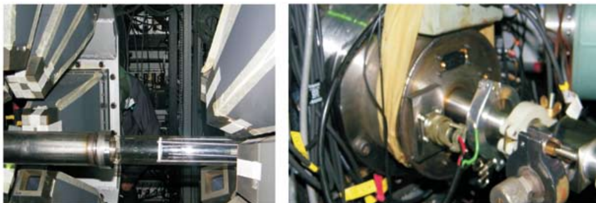
Fig. 2. Plunger mounted in INGA beam line showing the (left) front and (right) back views
