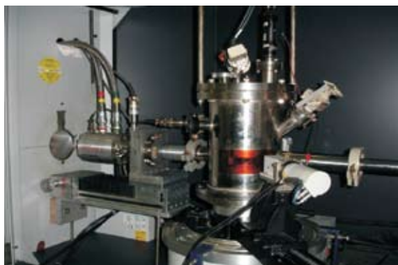
Fig. 1. Photograph of the closed cycle refrigerator installed with XRD system
