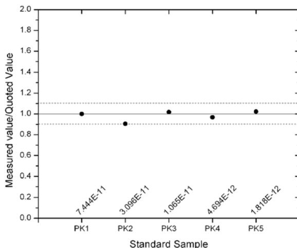
**Fig.1. Ratio of measured to quoted value for <sup>26</sup>Al measurement has been plotted for various concentrated standard samples. The ratio is close to one within ±10% for all the samples.**
