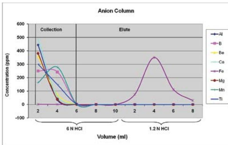
**Fig.2. Concentration of different elements after passing through the anion exchange column along with different volume of 6N and 1.2N HCl.**
