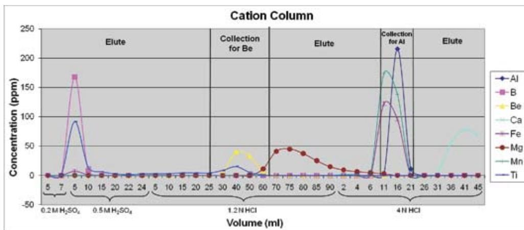
**Fig. 3. Concentration of different elements after passing through the cation exchange column along with different concentration of  $H_2SO_4$  and HCl.**
