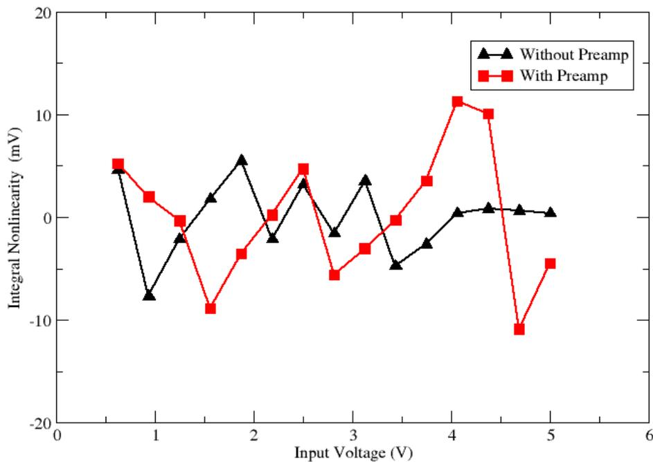
**FIG1: linearity error introduced by IUAC Charge sensitive preamplifier in ORTEC 572 amplifier output signal using Canberra pulser 8210.**
