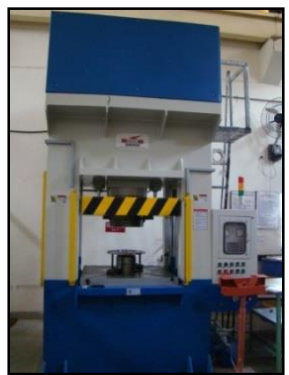
Cavity forming facility
