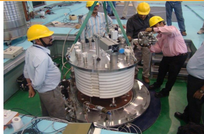
Lowering of cavity insert in VTS cryostat
