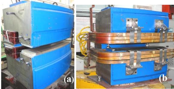
Figure 2: Pre-prototype dipole magnets (a). 0.5mm thick silicon steel laminated core (b). 1.5mm thick low carbon steel laminated core with water cooled coils
