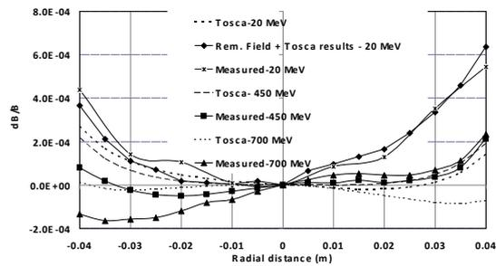
Figure 4: Comparison of measured and simulated radial field uniformities in the good field zone for low carbon steel magnet.
