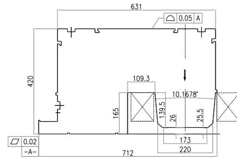
Figure 1: Half cross-section of dipole magnet in mm
