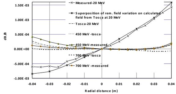
Figure 3: Comparison of measured and simulated radial field uniformities in the good field zone for CRNGO silicon steel magnet.
