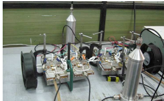
Figure 4: Photograph of 1 kW solid state RF system.
