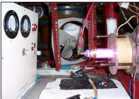
Figure 3: Photograph of RF source with D + plasma.
