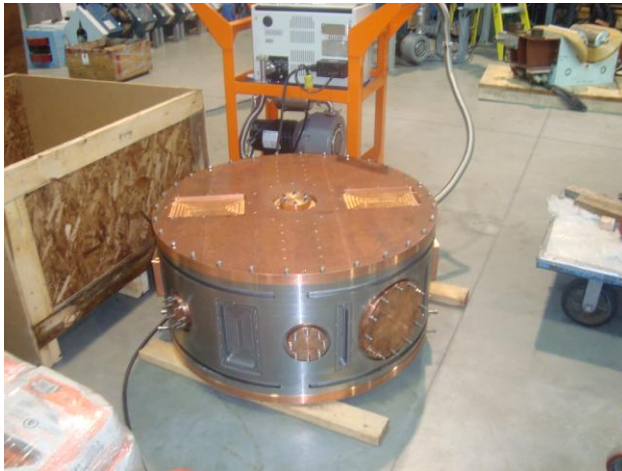
Figure 2. First DTL tank during vacuum test
