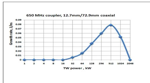
Figure 3: Multipacting growth rate
