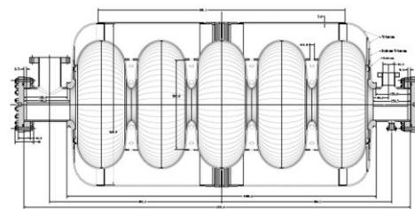
Figure 4: Layout of 650 MHz  $\beta=0.9$  cavity .
