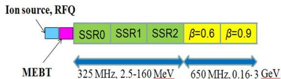
Figure 1: Acceleration scheme
