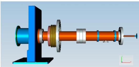
Figure 2: Power coupler for 650 MHz cavities.
