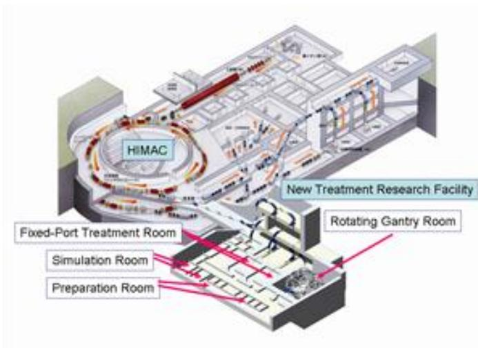
Fig. 4. Schematic view of the new treatment research facility.
