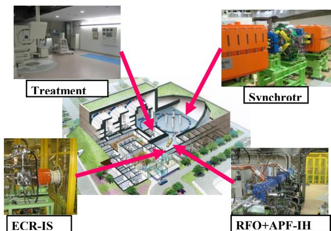
Fig. 3. Layout of the pilot facility constructed by GHMC.
