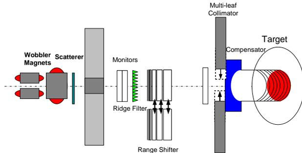
Fig. 2. Schematic drawing of the layer-stacking irradiation method.
