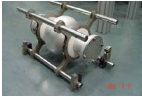
Figure 4 : Single cell cavity with mounting fixture for centrifugal barrel polishing machine.
