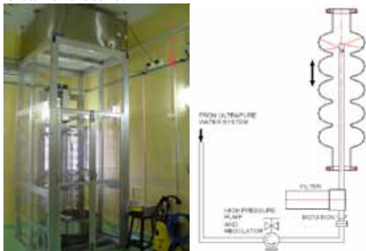
Figure 8 : Photograph of HPR set-up and working scheme
