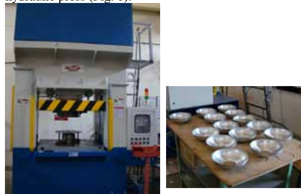
Figure 1 : Deep drawing 120 ton capacity hydraulic press and few deep drawn half cells of 1.3 GHz SCRF cavity
