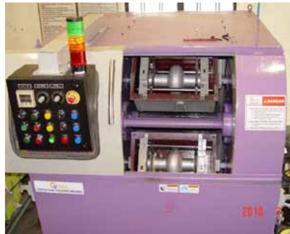
Figure 2 : Barrel polishing machine for Single cell 1.3 GHz SCRF cavity
