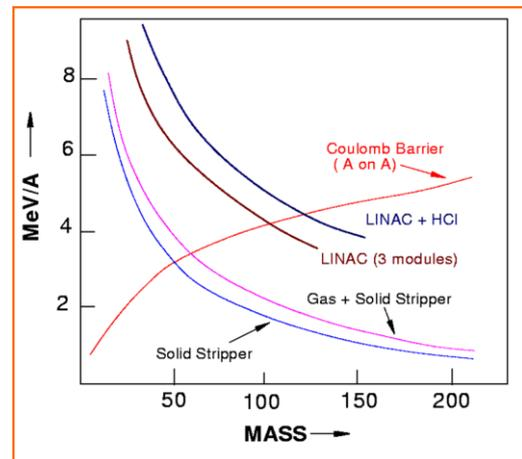
Figure 1. The energy per nucleon curve of the different ion species accelerated through Pelletron (light blue and pink), Pelletron + Linac (brown) and HCI + Linac (deep blue)
