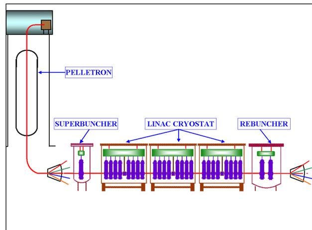
Figure 2. The schematic layout of Pelletron and Linac
