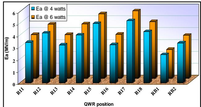
Figure 3. The accelerating field obtained at 4 and 6 watts of helium power. (R11-R18 and RB1-RB2 denote the eight and two QWRs of linac-1 and Rebuncher cryostat)
