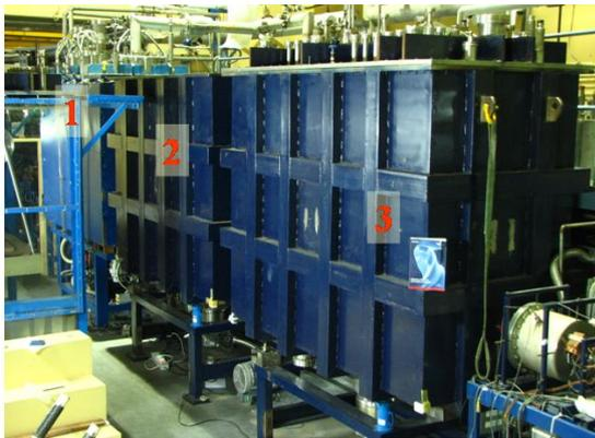
Figure 5. The remaining two cryostats 2 and 3 are installed in the beam line
