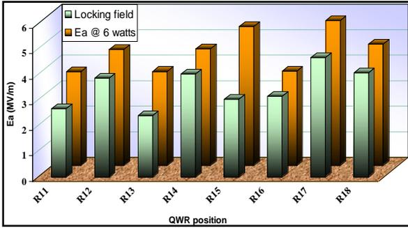
Figure 4. The accelerating field in phase lock condition
