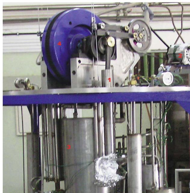
Figure 2: Photograph showing expansion engine developed at RRCAT. 1. Cryogenic Expander, 2. Work extraction mechanism, 3. 1<sup>st</sup> heat exchanger, 4. Flywheel
