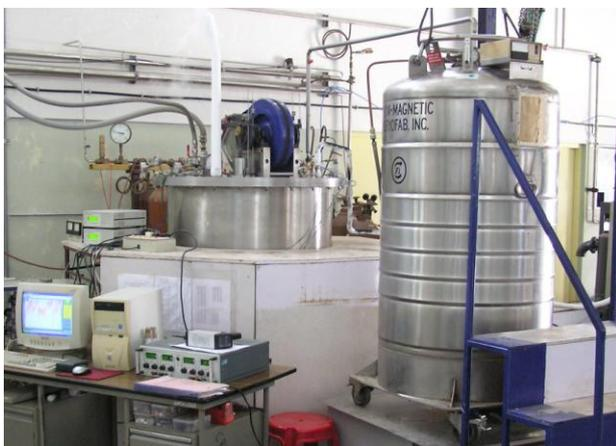
Figure 4: Photograph shows Helium Liquefier developed at RRCAT
