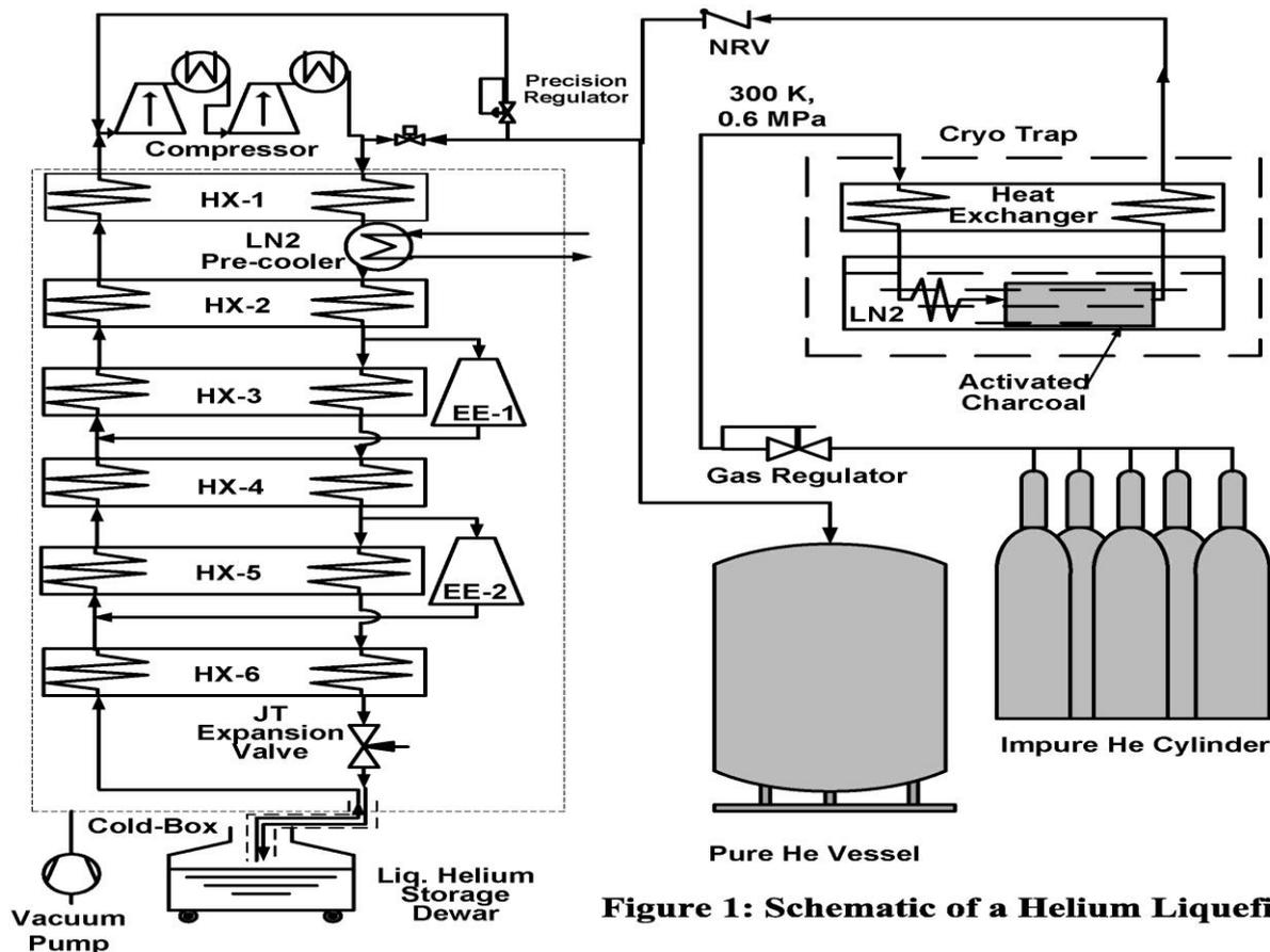
Figure 1: Schematic of a Helium Liquefier
