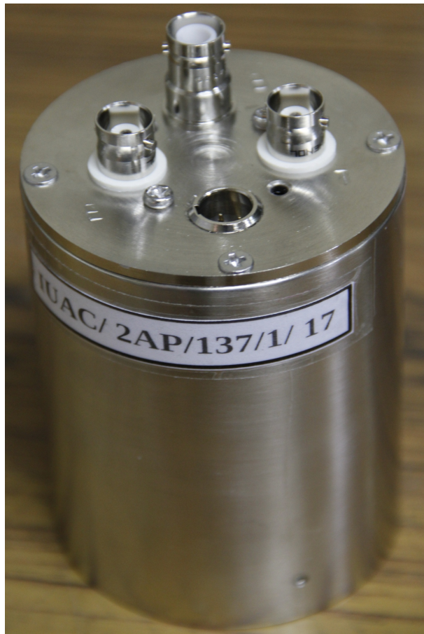
Fig: Photo of PMT base with High voltage divider network and Charge sensitive Preamplifier
