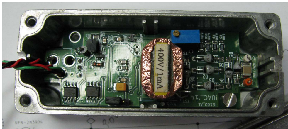
Figure 7: Internal view of power supply unit
