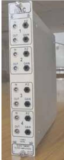
**Fig. 2. Quad Timing Filter Amplifier module**
