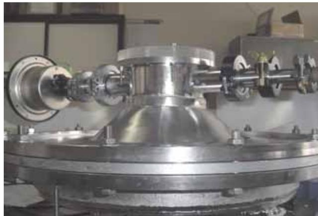
**Fig.1 SS target(conical) and detector chamber (below) with Aluminum foil flange in between**
