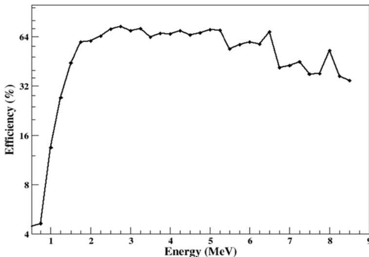
Fig. 4.1.5 Efficiency spectrum at 300 keV threshold
