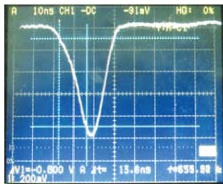
Fig. 4.1.3 Timing signal from MWPC
