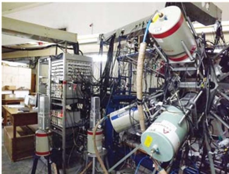
Fig. 4.2.1 Clover detectors being tested in GDA beam line area
