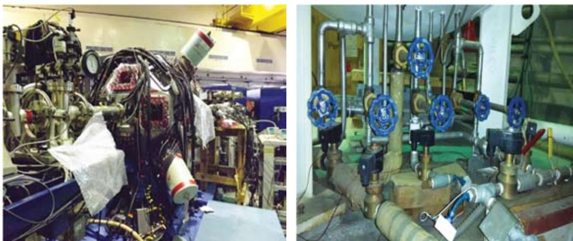
Fig. 4.2.2 (a) Clover and ACS detectors mounted in INGA support structure
