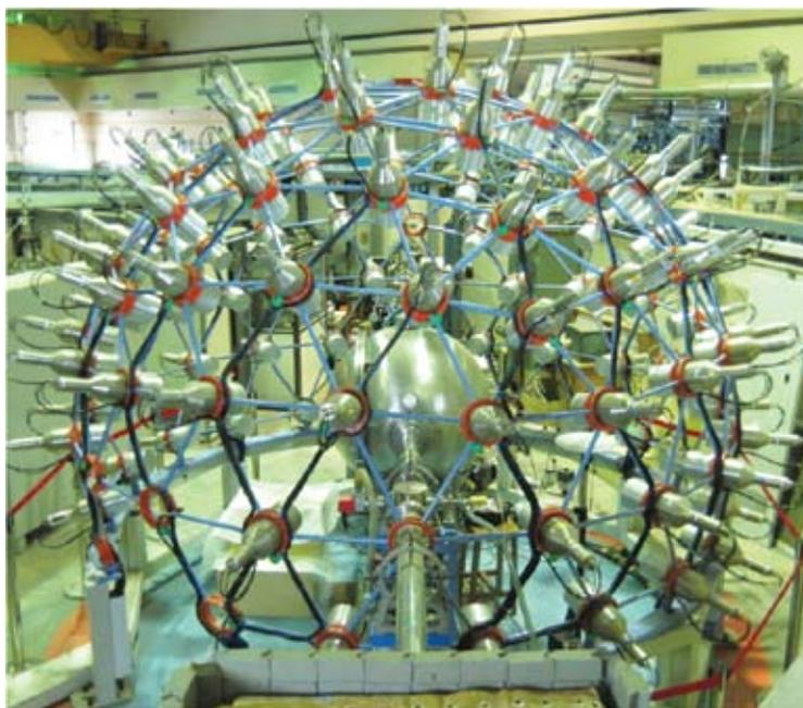
Fig. 4.1.2 Neutron Detector array facility installed in Beam Hall II at IUAC
