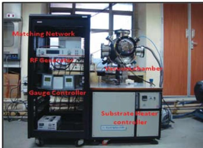
Fig.4.4.2 Photograph of the RF sputtering system for preparation of oxide thin films
