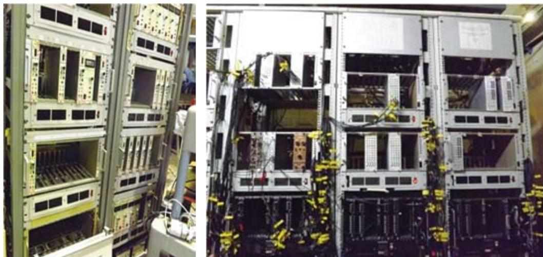
Fig. 4.2.3 (a) High voltage power supplies and (b) Clover modules and ADCs being tested
