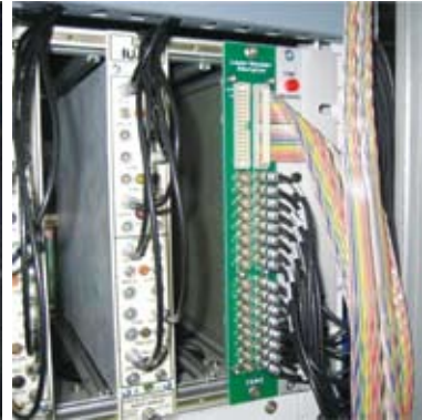
Fig. 3.1.12 Lemo to Header Adapter installed in NAND Exp. set-up
