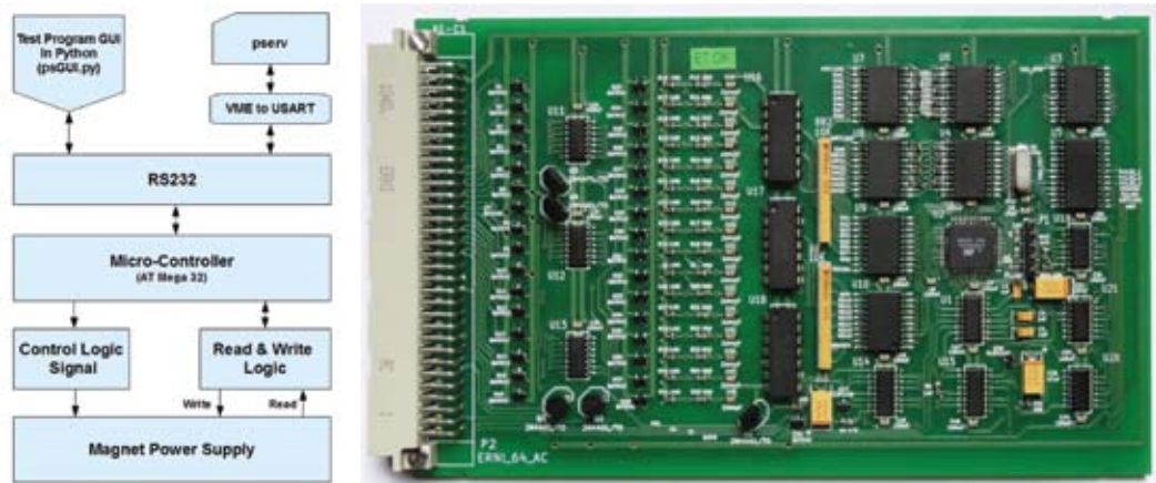
Fig. 3.1.4 (a) Schematic for USART interface (b) Custom hardware card for magnet power supply
