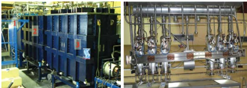
Fig. 1. The first picture shows the three accelerating module of the Superconducting Linear accelerator of IUAC. The second picture shows the last linac accelerating module being installed with six resonators.
