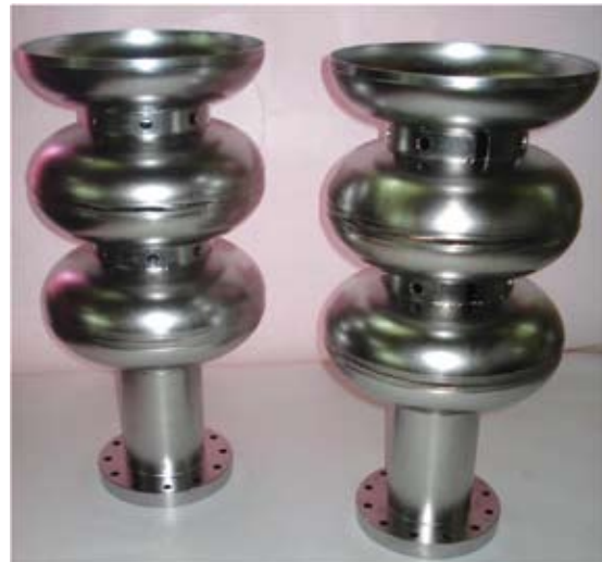
Fig. 4. The two halves of the 5-cell TESLA-type Cavity.
