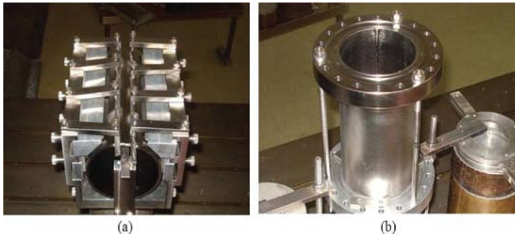
Fig. 6. (a) Electron beam welding setup for the seam welding of the end tube, (b) setup showing the electron beam welding of the tube to Nb-Ti flange.
