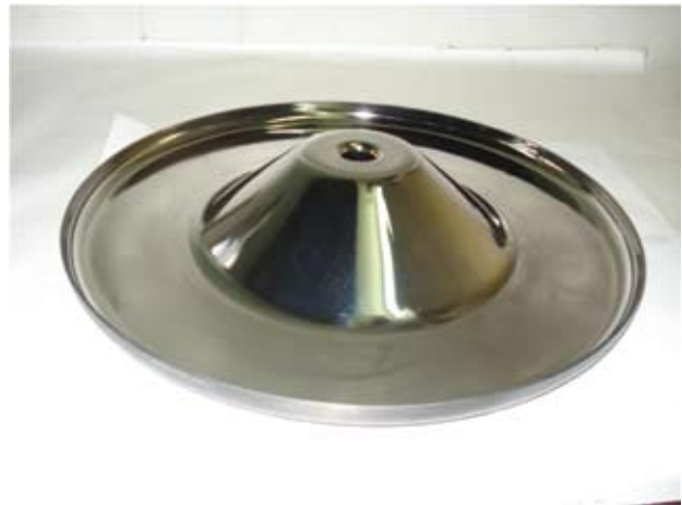
Fig. 1. RF surface of an electropolished End Wall for the Single Spoke Resonator -SSR1.
