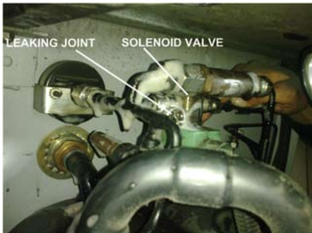
Fig. 1. Location of the solenoid valve and leak location in the extraction cryo-cooler using soap solution.
