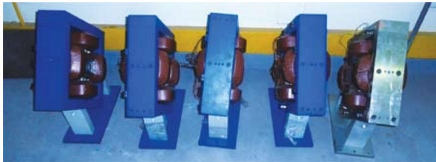
Fig. 25 Fabricated and tested magnetic quadrupoles
