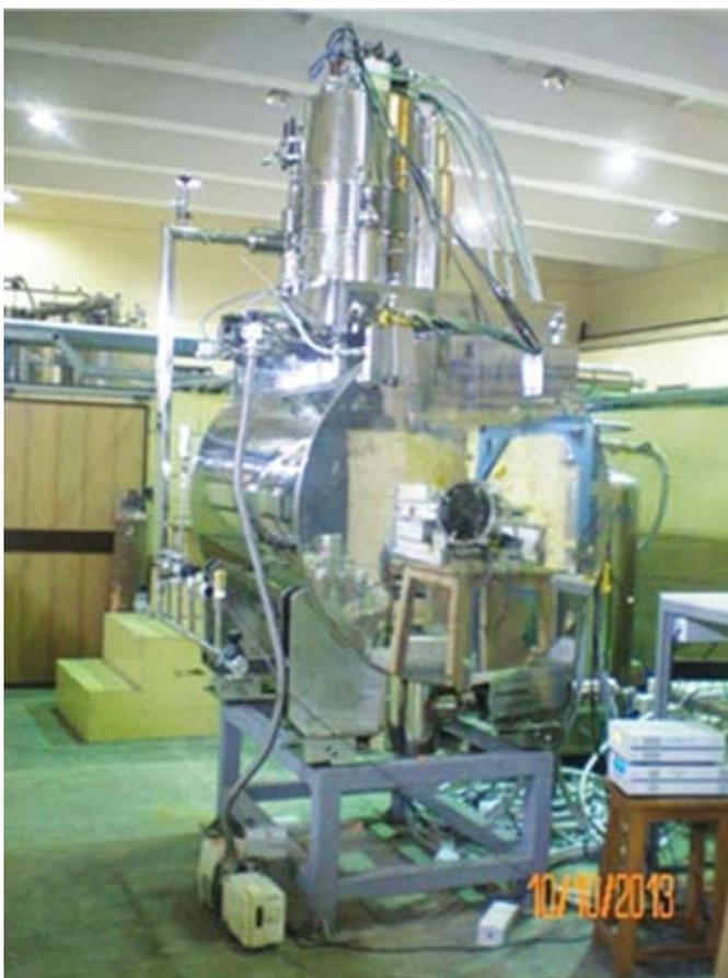
Fig. 28 Superconducting Quadrupole Doublet Magnet
