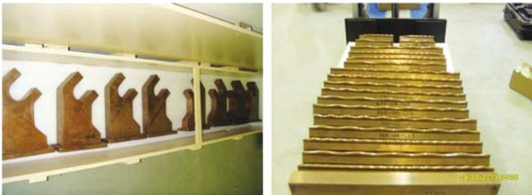
Fig. 17. Stem supports and vanes for the RFQ accelerator.
