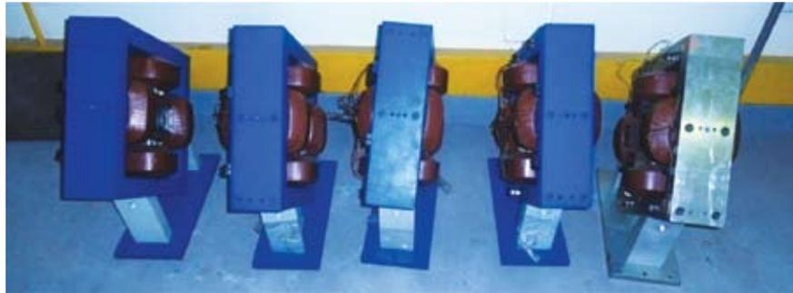
Fig. 25 Fabricated and tested magnetic quadrupoles
