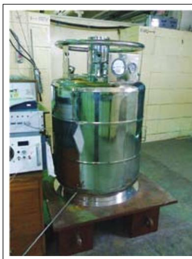
Fig. 31. LN<sub>2</sub> dewar with cryocooler
