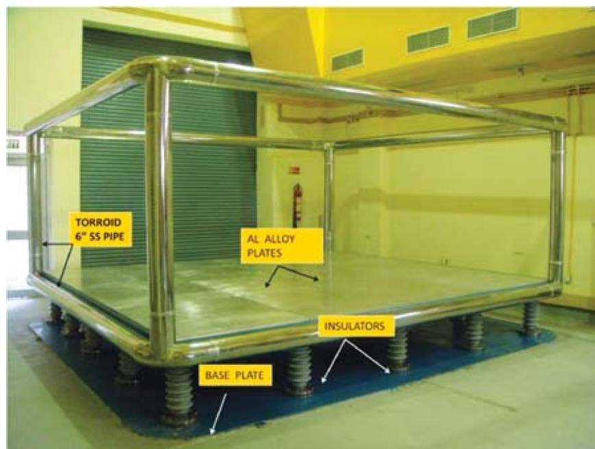
Fig. 9. View of 100 kV high voltage platform installed in beam hall III
