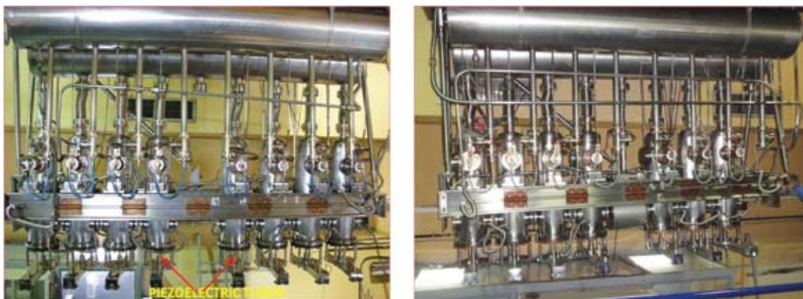
Fig. 1. The second (a) and third (b) accelerating linac modules with the gas based mechanical tuning system replaced by the piezo actuator based tuning mechanism.
