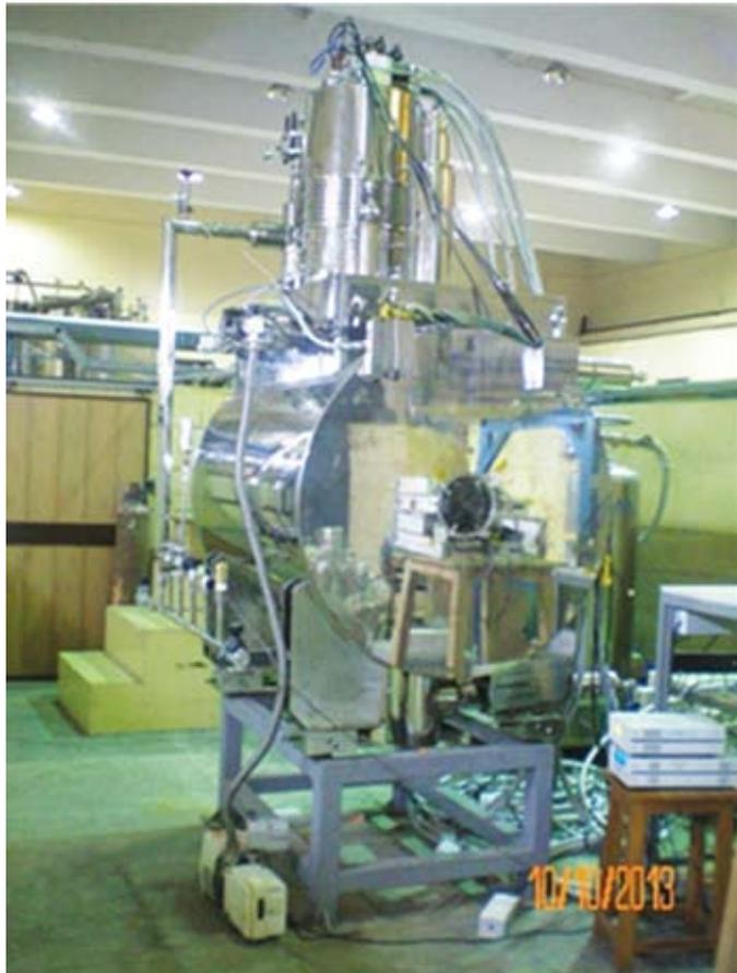
Fig. 28 Superconducting Quadrupole Doublet Magnet
