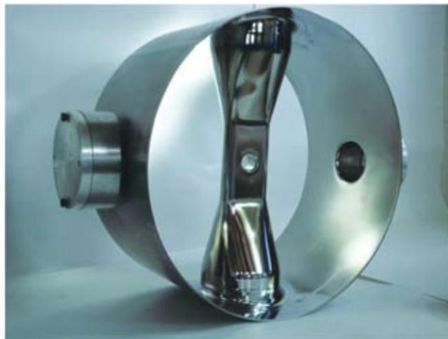
Fig. 4: Spoke assembly after electron beam welding to the outer niobium shell.
