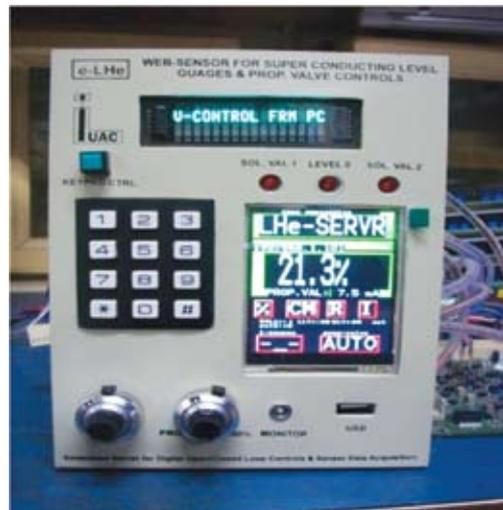
**b) LN2 level servers for Capacitive level sensors**
