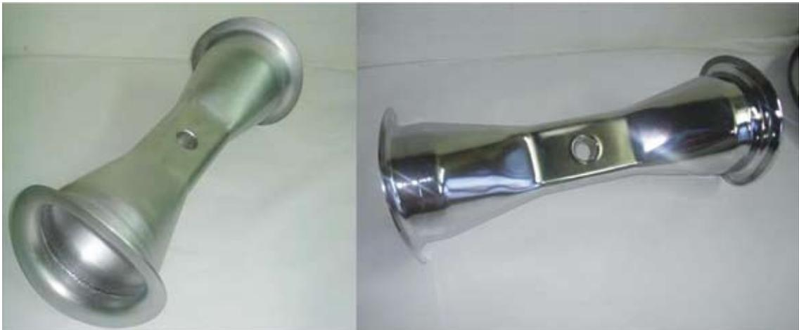
Fig. 3: Spoke assembly after completion but before electropolishing (left) and electropolished spoke assembly (right) ready for attachment to the Shell.
