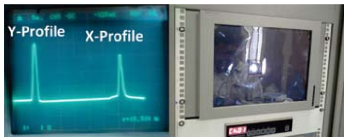
Fig. 2: a) A typical profile of 215 keV O + beam b) Beam spot on the target
