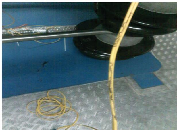
Fig. 1.3.5 A view of the damaged fiber optic cable
