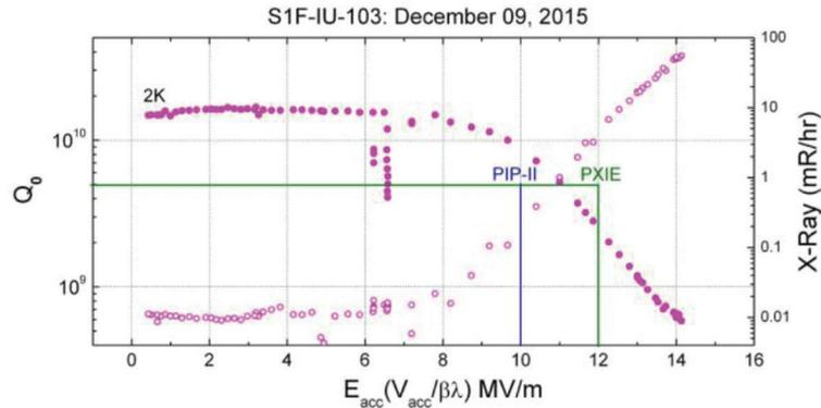
Fig. 1.2.3 Performance of IUAC built SSR1 Niobium Spoke Resonator S103 at 2K
