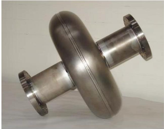
Fig. 1.2.4 First 650 MHz,  $\beta=0.61$  niobium single cell low beta cavity
