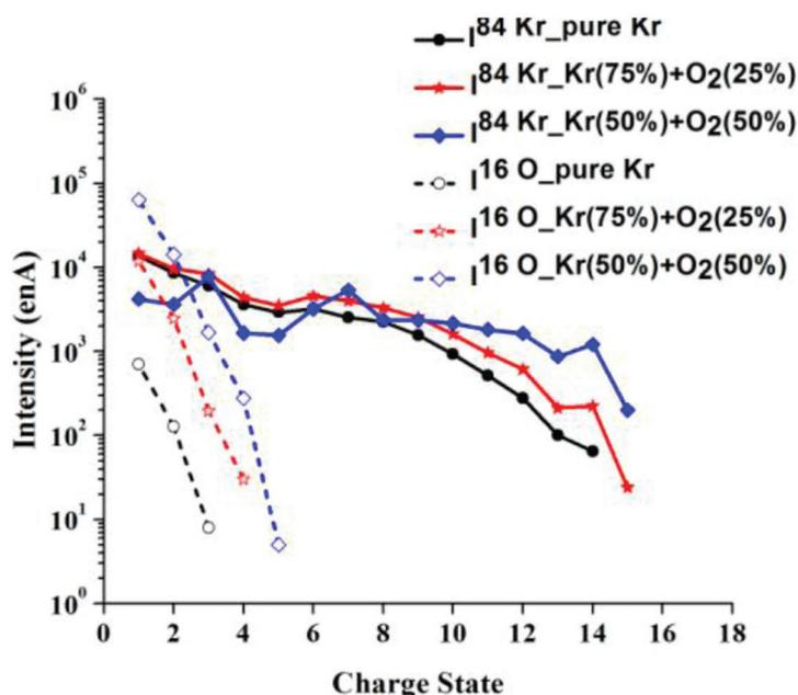
Fig. 1.3.1 A typical charge state distribution of the krypton showing the influence of the oxygen mixing on the higher charge states.
