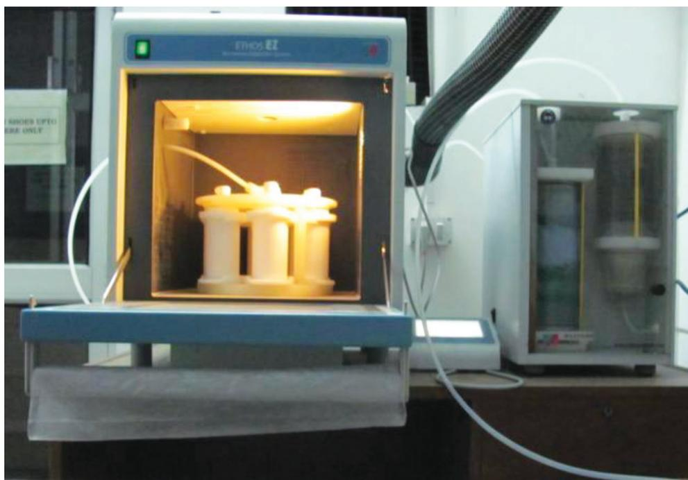
Fig. 1.5.1 Microwave digestion system at IUAC
