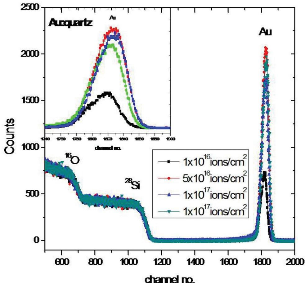
Figure 1.1.4: RBS spectra for 70keV Au- ion implantation in fused quartz substrate with ion fluence from  $1 \times 10^{16}$  ions/cm<sup>2</sup> to  $1 \times 10^{17}$  ions/cm<sup>2</sup>.
