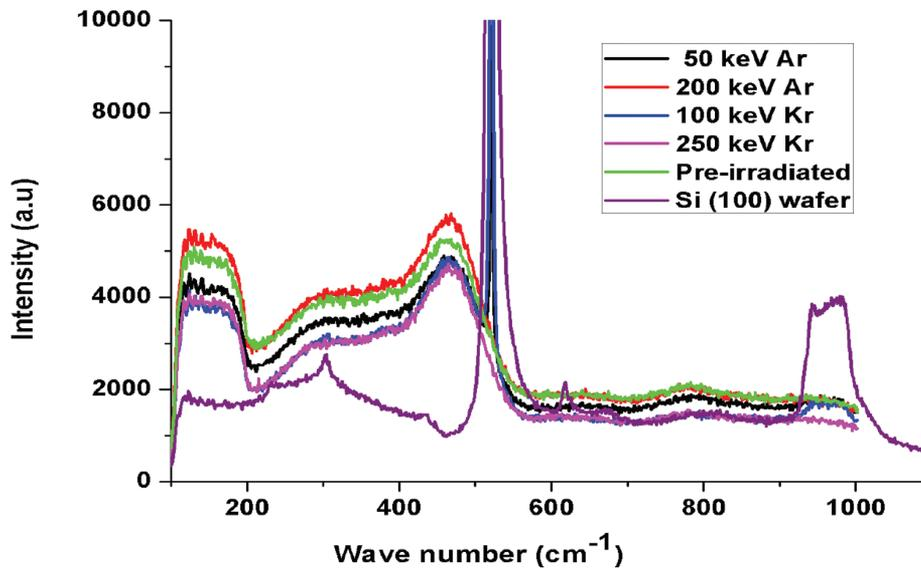
Fig. 1.3.4 Re-crystallization of a-Si by the irradiation of 100 keV Kr ions
