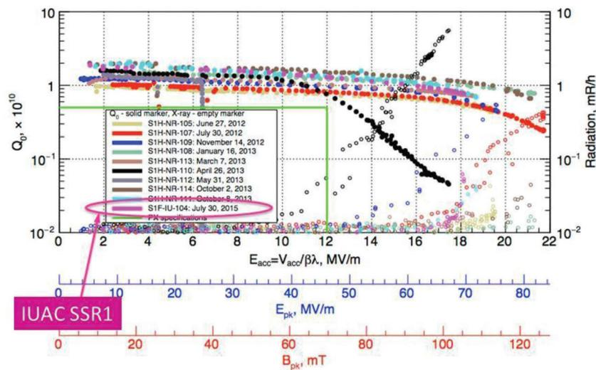
Fig. 1.2.2 Performance of IUAC built SSR1 Niobium Single Spoke Resonator S104 at 2K along with several other resonators tested at Fermilab
