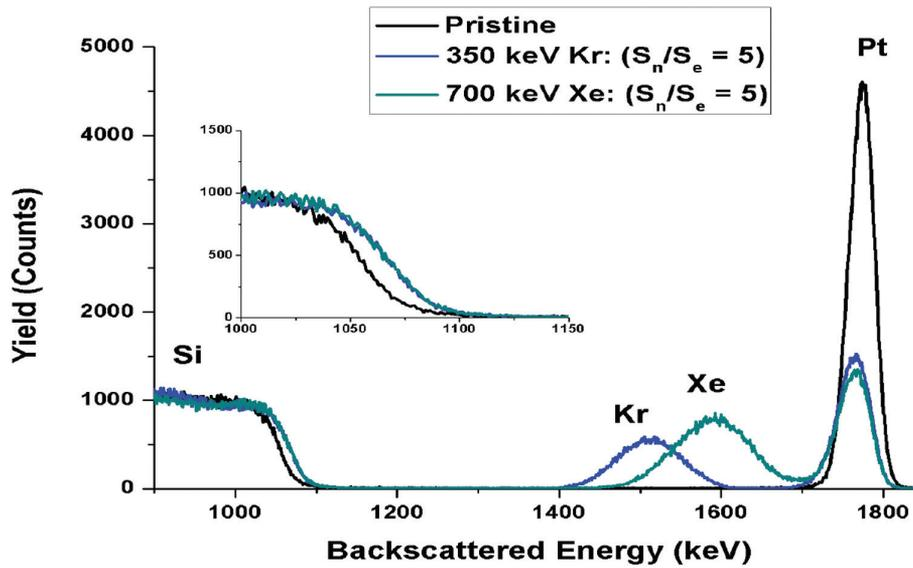
Fig. 1.3.3 The RBS spectra of Pt:Si thin films irradiated with low energy Kr and Xe beams. The zoom image of Si edge is shown in the inset.
