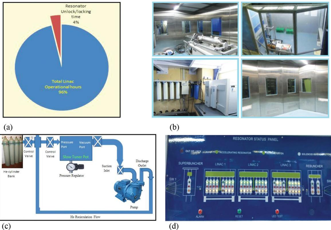
Fig. 1.2.1 (a) Pie chart for the linac up-time, (b) clockwise - the high pressure water rinsing facility, the resonator assembly room, the linac servicing area and the RO/Super-Q plant, (c) the closed loop helium gas circulation system for the mechanical tuner of SC resonator and (d) the status display used during linac operation.
