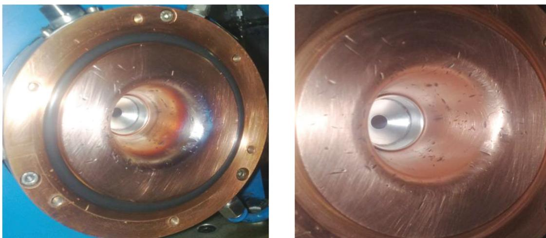
Fig. 1.3.6 A view of ionization chamber; left) before cleaning, right) after cleaning
