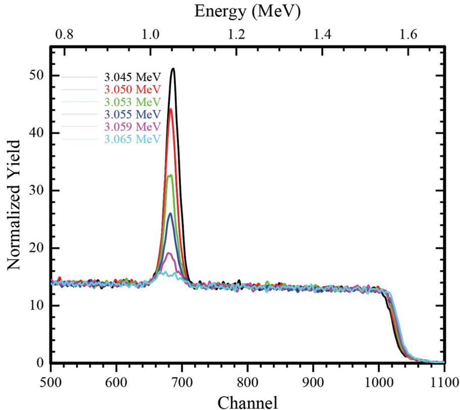
Fig 1.4.1 RBS Spectra of Oxygen resonance on Silicon substrate with increasing energy
