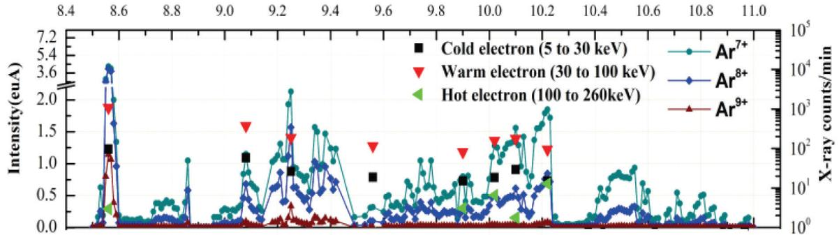
Fig. 1.3.2 The effect of frequency tuning on the intensity of highly charged argon ions. The electron energy distribution deduced from Bremsstrahlung spectra is also given.
