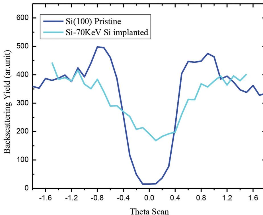
Fig. 1.4.2 Angle Scan of Si single crystal in comparison with surface amorphized by ion implantation.
