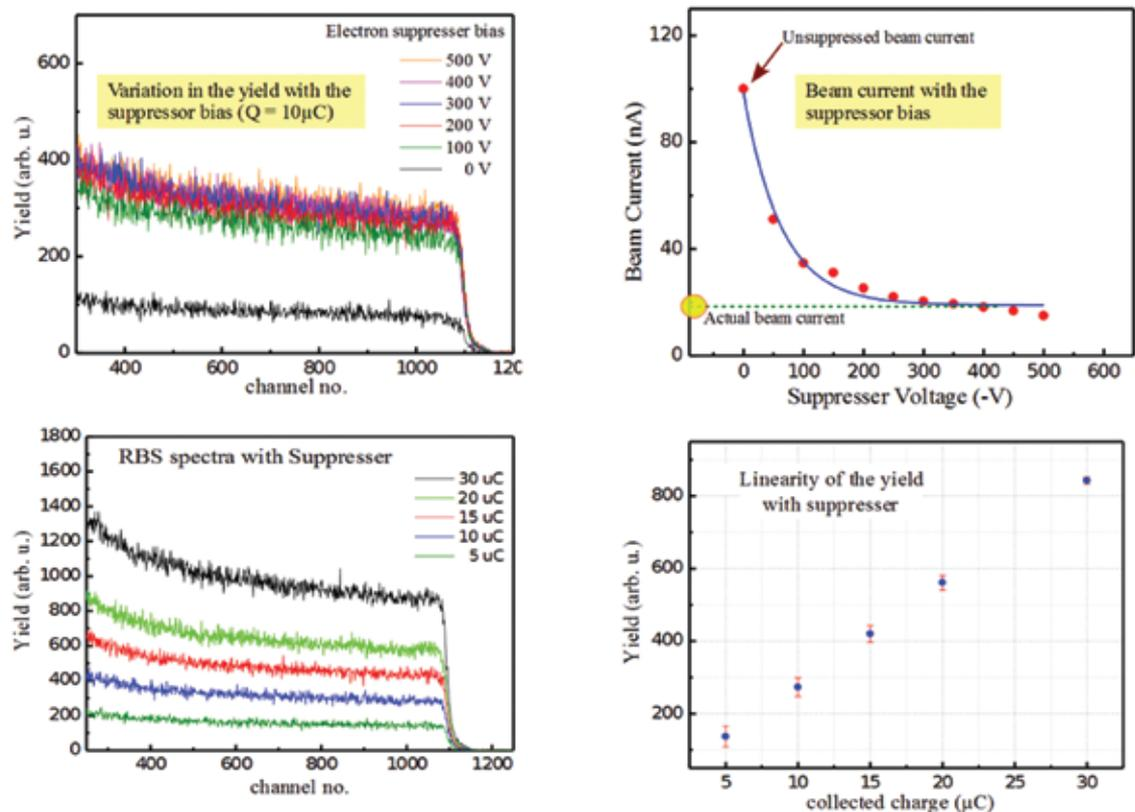
Fig. 10 Testing of electron suppressor and RBS spectra using Si samples.
