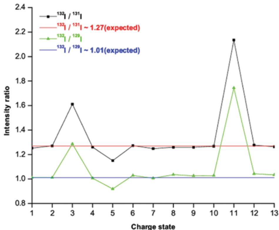
Fig. 6 Intensity ratio of xenon isotopes ( $I^{132}/I^{131}$  and  $I^{132}/I^{129}$ ) for different charge states. The red and blue curves are expected ratios of  $I^{132}/I^{131}$  and  $I^{132}/I^{129}$  in the natural xenon.
