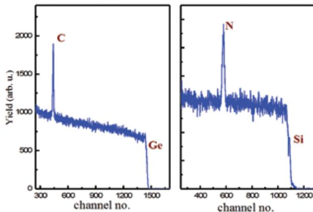
Fig. 9 Typical resonant RBS spectra for the analysis of C and N in different samples.
