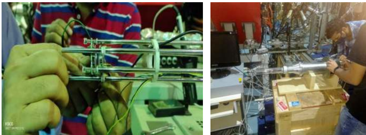
Fig. 4.2.3.1: Plunger target-stopper assembly (left) and assembled plunger device inside the scattering chamber made of glass and with a diameter of 4 cm (right).
