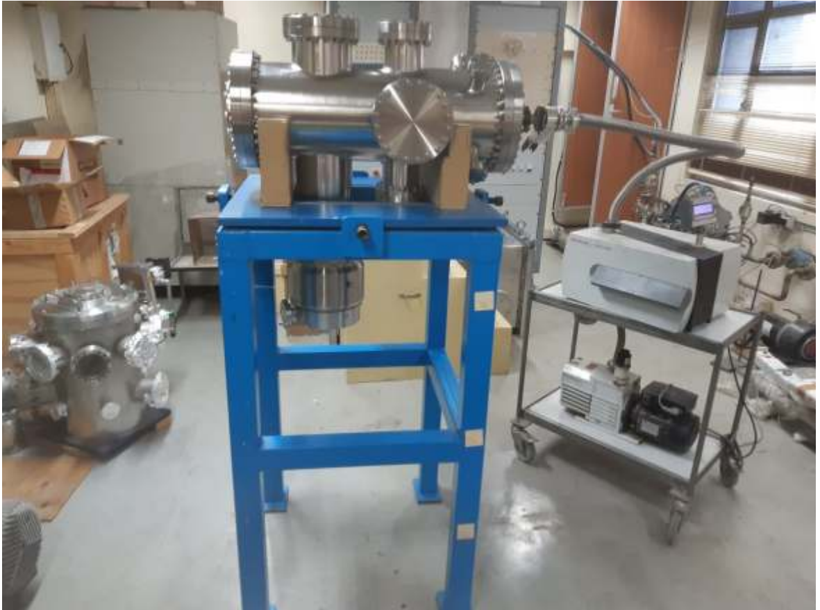
Fig 5. Picture of the ultra-high vacuum chamber during vacuum leak tests.
