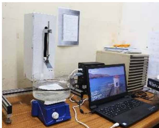
Figure 1: Dip coating machine for stripper foil floating
