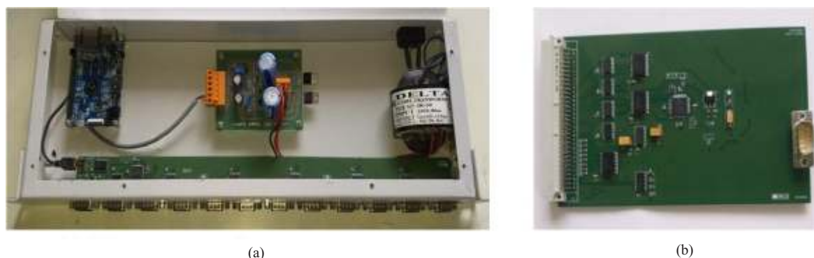
Fig 4: (a) RS-232 Server Controller (b) RS-232 to IGOR Convertor Card
