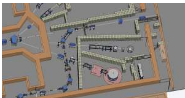
Fig 2: Beam line of HCI (in beam hall I) and proposed shielding modifications
