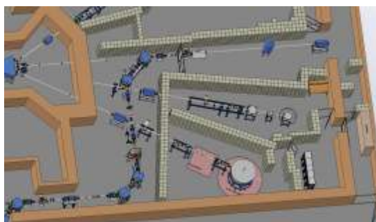
Fig 2: Beam line of HCI (in beam hall I) and proposed shielding modifications
