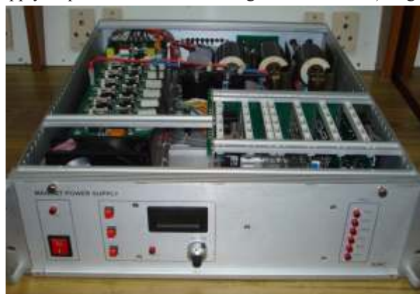
Fig 1: In-house Developed Low Current bipolar Power Supply (LCPS)
