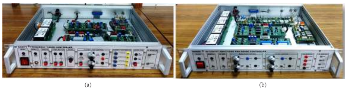
Fig 3: (a) Amplitude and Phase Control Unit and (b) Frequency tuner control unit
