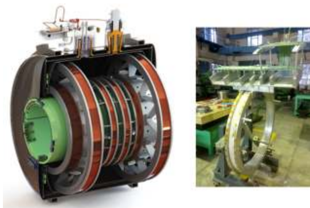
Fig. 3.1.2.4 (a) The cut -view of the superconducting MRI magnet and, (b) the one-twelfth section of bobbin integrated on a prototype bobbin stand.
