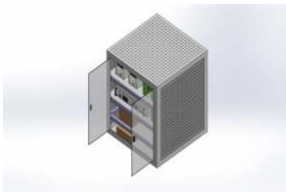
Fig 7. Model of modified 40 kV high voltage cabinet.
