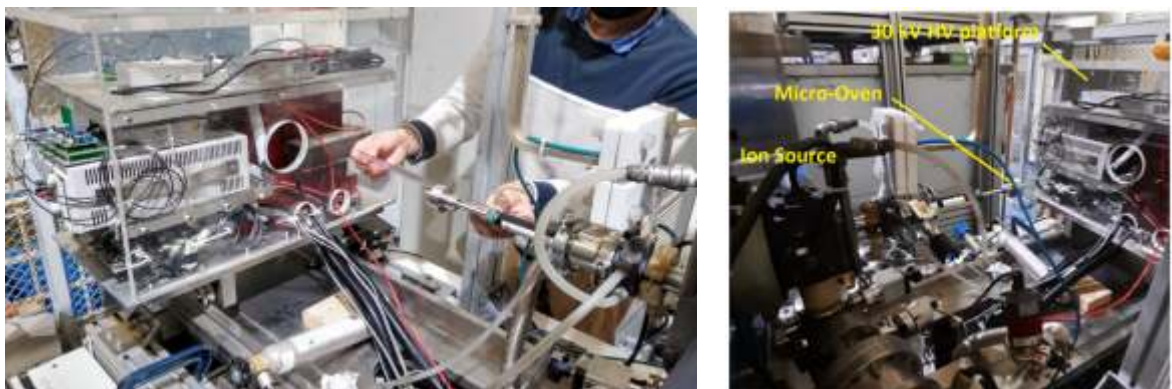
Fig 6. (Left)View of the 30 kV high voltage platform; (Right) View of installed micro-oven.
