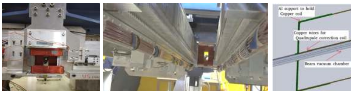
Fig 2. Images show the end correction coils, long coils and the schematic of the quadrupole correction coils.
