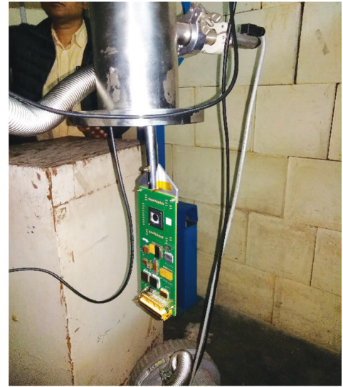
Fig. 1: DUT card mounted on target ladder
