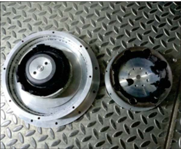
Figure 3: Damaged rubber coupler of Unit 23 - 24.
