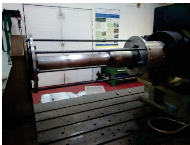
Figure 3a: Tack weld of loading arm to drift tube.
