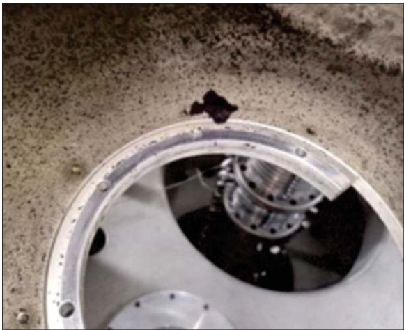
Figure 4: Dust inside accelerator due to damaged rubber coupler.
