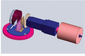
Fig. 1 : Focal Plane Setup : MWPC followed by Silicon & Clover Detecters
