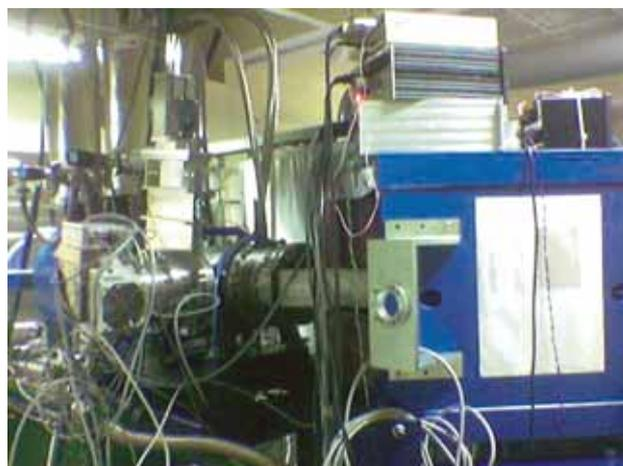
**Fig. 1. PKDELIS ECR ion source and Low Energy Beam Transport system (LEBT)**
