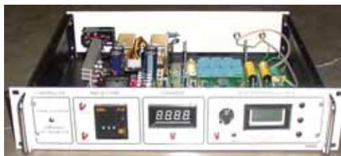
**Fig. 10. Controller for Spark Counter and Beta Ray Spectrometer**
