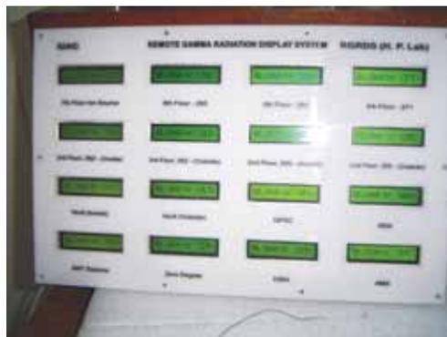
Fig. 13. Digital gamma radiation display at Pelletron control room
