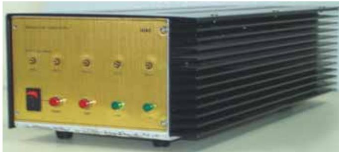
**Fig. 9 : Pre-amplifier Power Supply**
