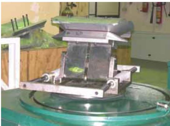
**Fig. 10A. Flipping mechanism of winding machine**
