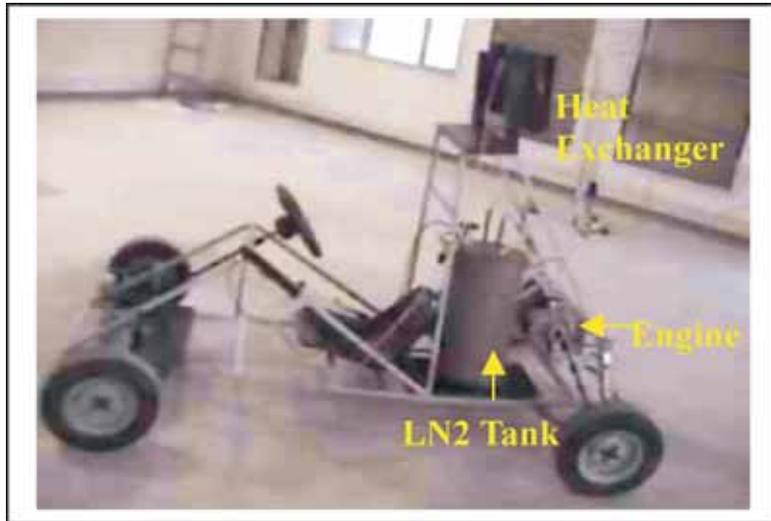
**Fig. 10. Picture of LN2 driven demo-car**
