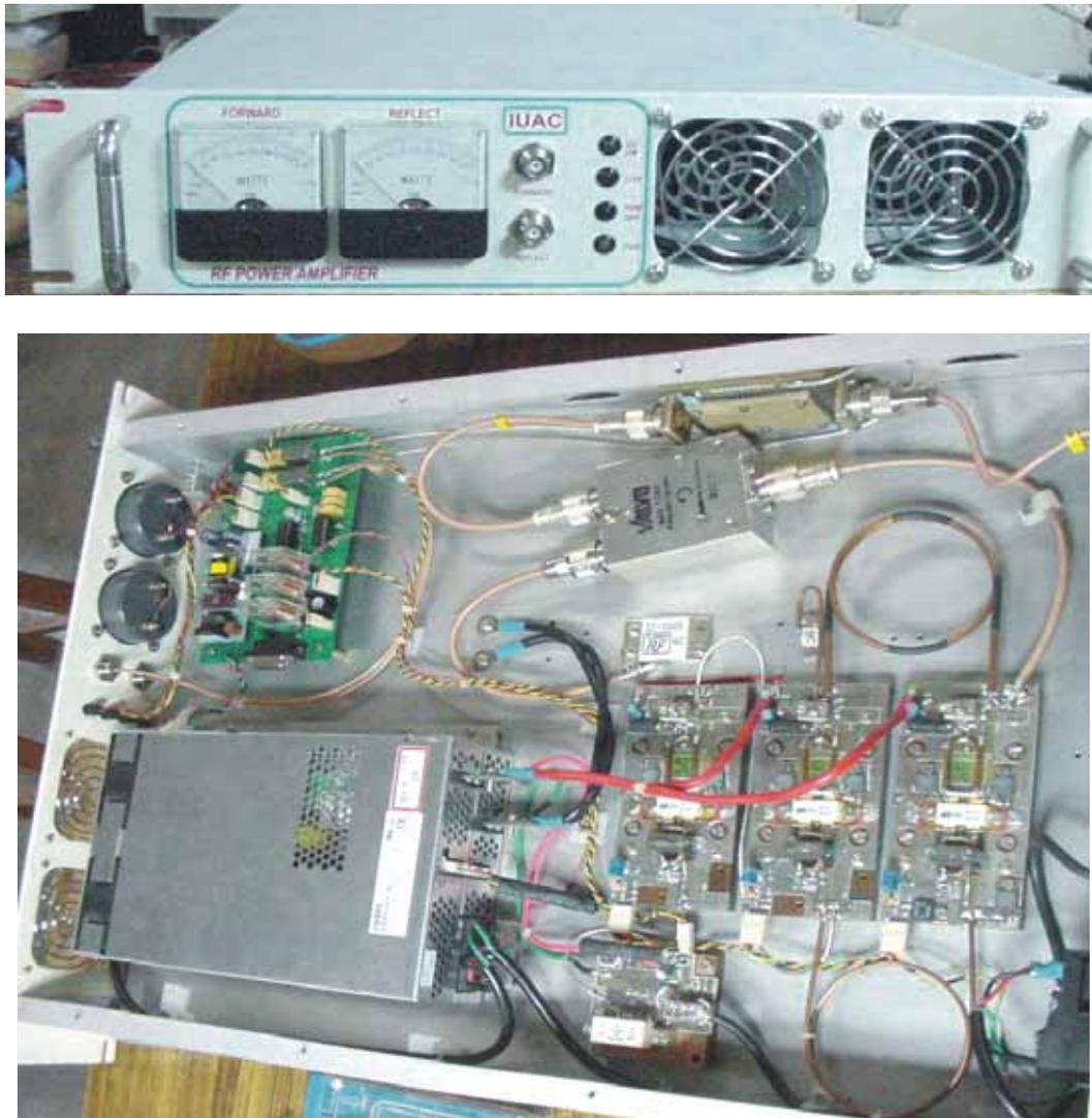
**Fig. 1. 400Watts VHF Power amplifier**
