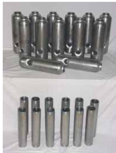
**Fig. 1(b) Drift Tubes (top) & Loading Arms (bottom)**
