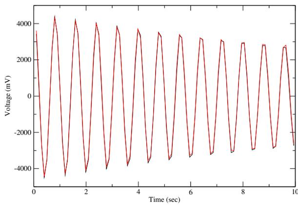
Figure 4.23: Decaying oscillations
