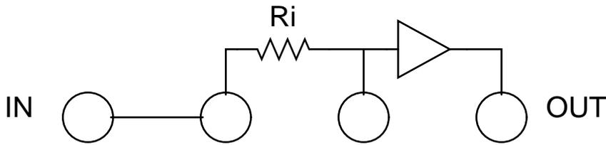
Figure 3.4: Inverting Amplifier
