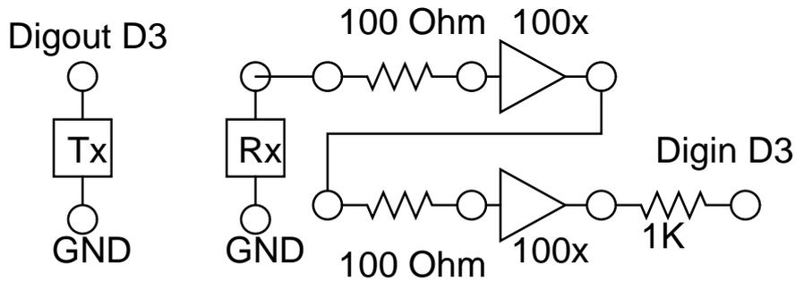
Figure 4.19: Piezo Transceiver setup measuring velocity of sound
