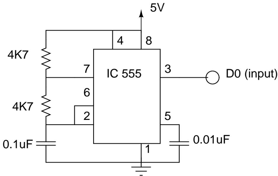
Figure 4.26: 555 oscillator circuit
