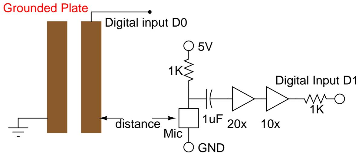
Figure 4.20: Velocity of sound by microphone
