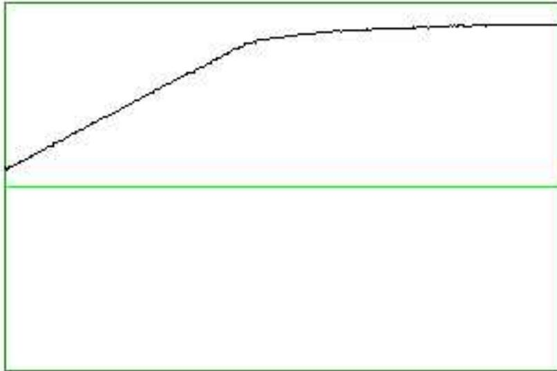
Figure 4.7: Linear charging.  $R = 1 \text{ K}\Omega$  ,  $C = 1 \text{ }\mu\text{F}$
