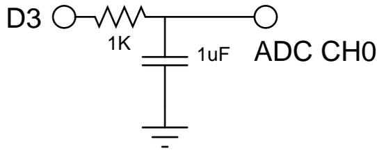
Figure 4.4: Circuit to study Capacitor
