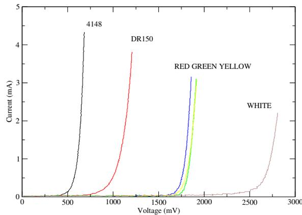
Figure 4.9: Diode Characteristics
