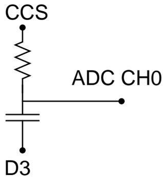
Figure 4.6: Linear Charging of Capacitor
