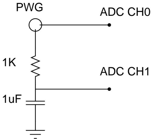
Figure 4.10: Integration circuit
