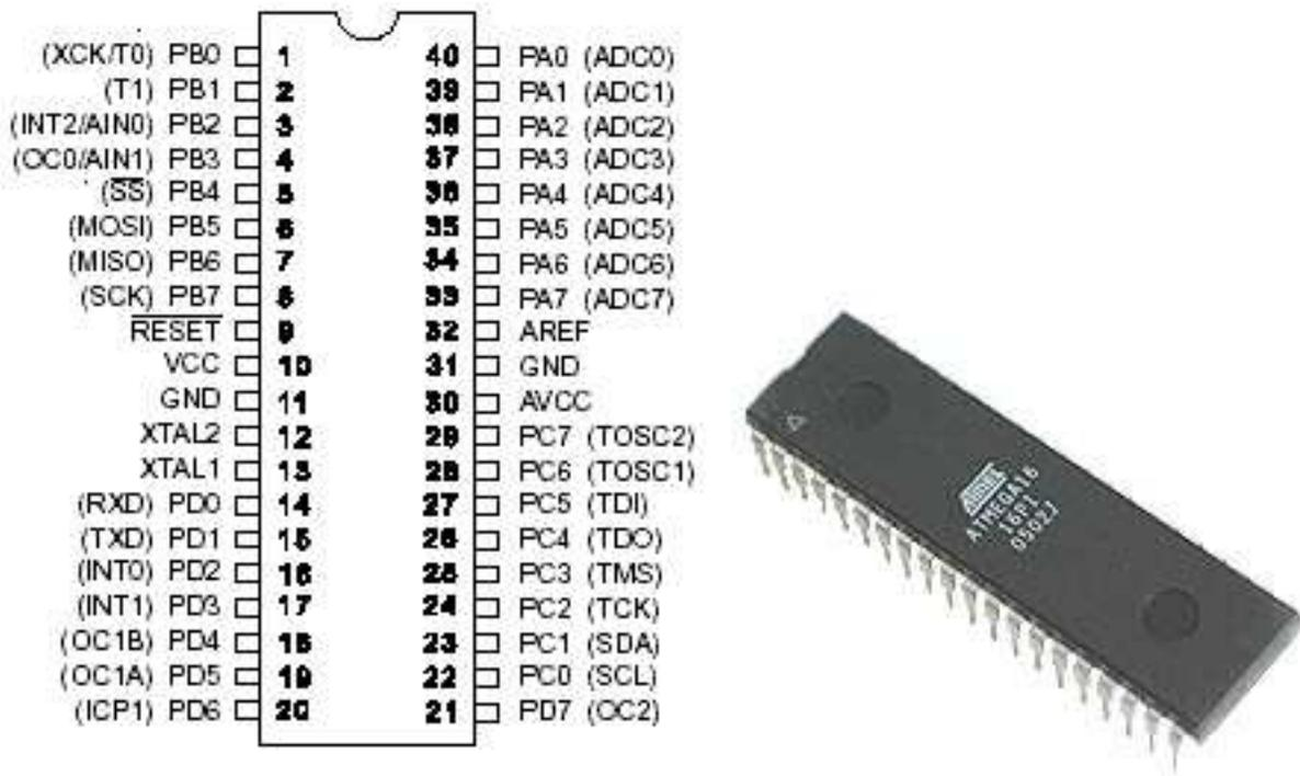
Figure 5.1: ATmega16 . Pin diagram and DIP package
