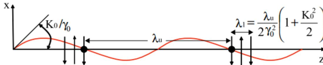
FIG. 2. (Color) After an electron (black dot) travels one undulator period  $\lambda_u$  of the sinusoidal trajectory (in red), a plane wave (represented by alternating vertical arrows) overtakes the electron by one resonant wavelength  $\lambda_1$ . Thus, the undulator radiation carrying this resonant wavelength can exchange energy with the electron over many undulator periods.
