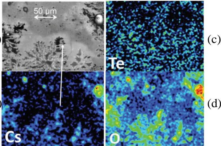
EDX analysis of Cu(Cs<sub>2</sub>Te)<sub>13</sub> cathode showing the distribution of Cs (caesium), O (oxygen) and Te (Tellurium). The SEM reference picture (with back scattered electrons) is in the upper left corner.
