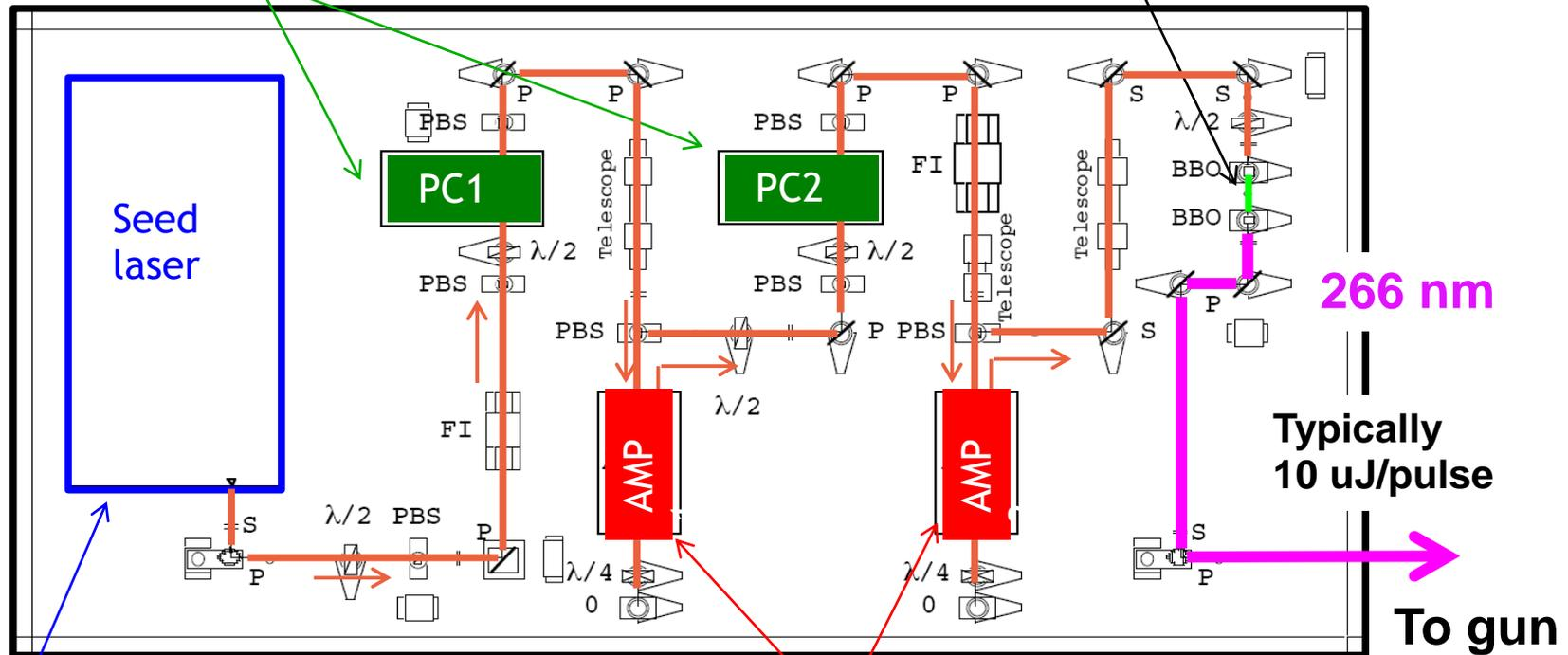
TBP, 357MHz mode-locked pulse laser
