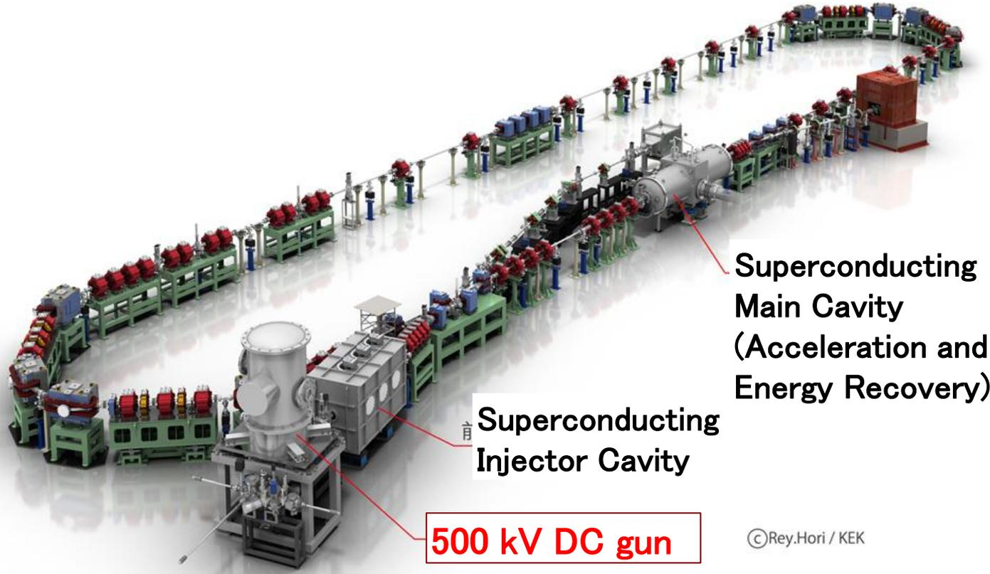
Superconducting Main Cavity (Acceleration and Energy Recovery)
