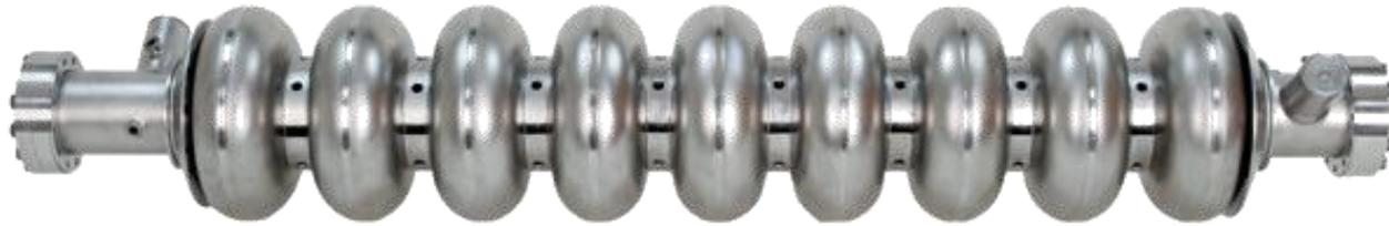
**9-cell Nd superconducting cavity**
